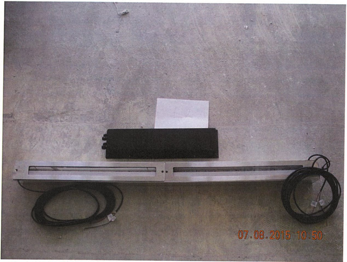
'L2' Luminaire in DBB Box and Power Supply
