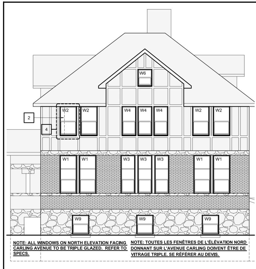
NOTE: ALL WINDOWS ON NORTH ELEVATION FACING CARLING AVENUE TO BE TRIPLE GLAZED. REFER TO SPECS. / NOTE: TOUTES LES FENÊTRES DE L'ÉLÉVATION NORD DONNANT SUR L'AVENUE CARLING DOIVENT ÊTRE DE VITRAGE TRIPLE. SE RÉFÉRER AU DEVIS.
