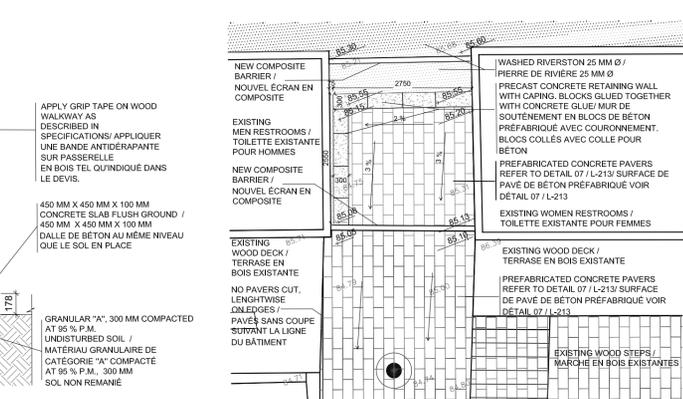
10 RETAINING WALL AND STORAGE UNIT / MUR DE SOUTÈNEMENT ET RANGEMENT scale / échelle 1:70
