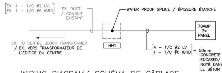
WIRING DIAGRAM / SCHÉMA DE CÂBLAGE
