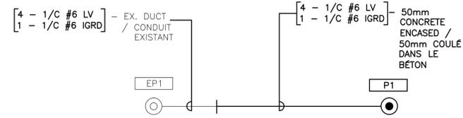
WIRING DIAGRAM / SCHÉMA DE CÂBLAGE
