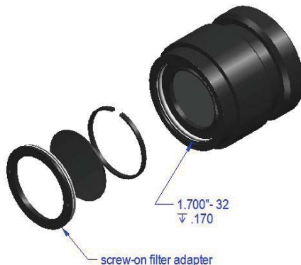
Figure 10: Screw-on filter adapter with the objective inside wall threads 6. ADDITIONAL FEATURES
