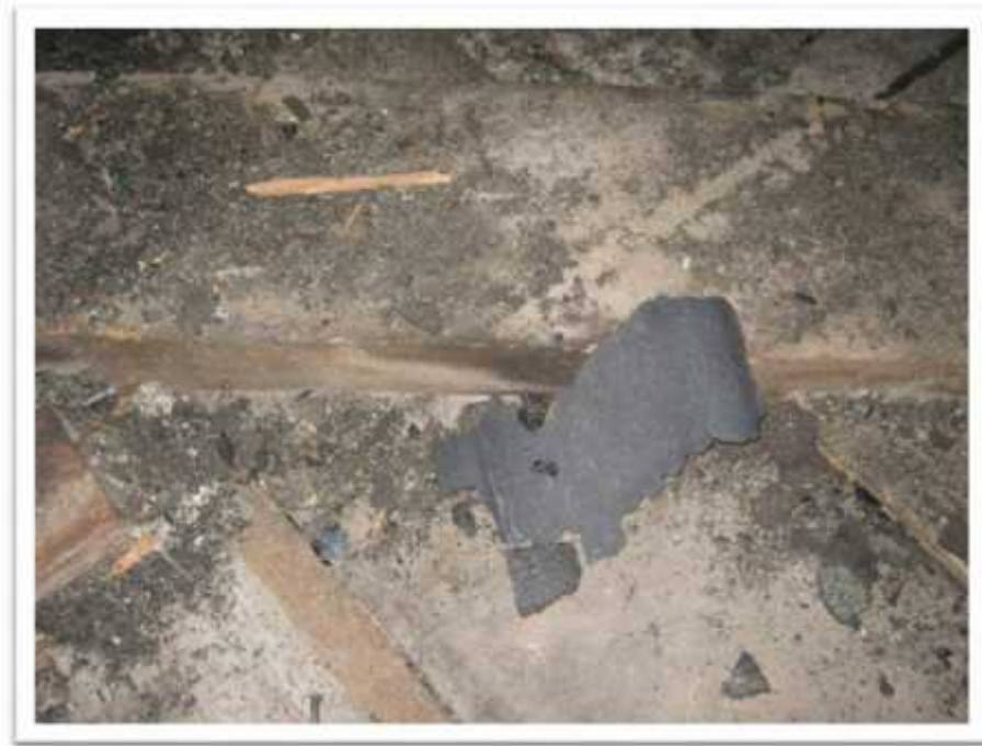
Photo 17: Tar paper debris in the attic (Sample 243867-13A) contains 1% chrysotile asbestos.
