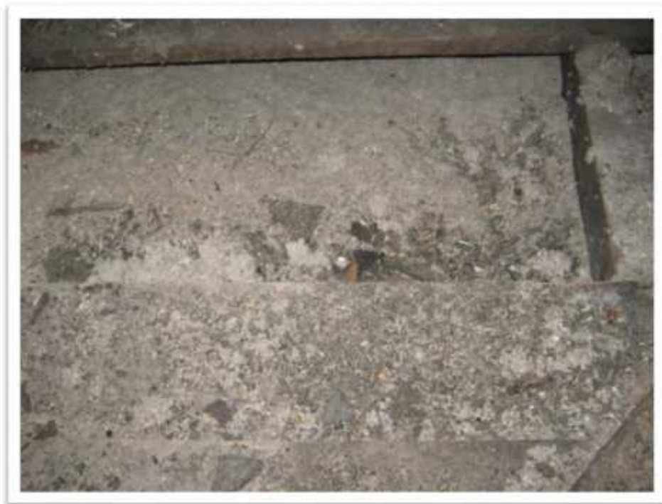
Photo 16: Roof shingle debris sampled in the attic does not contain asbestos (Samples 243867-12A-C).
