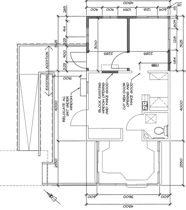
NOTE: WINDOWS AND DOOR OPENINGS TO PROVIDE A CLEAR PASSAGE OF 813mm (MINIMUM). DOOR HARDWARE TO BE LEVER TYPE TYPICAL.
