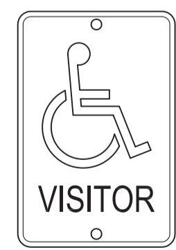
SIGN TYPE 'A' BARRIER FREE PARKING SIGNAGE COLOUR: BLUE ON WHITE PROVIDE 1
