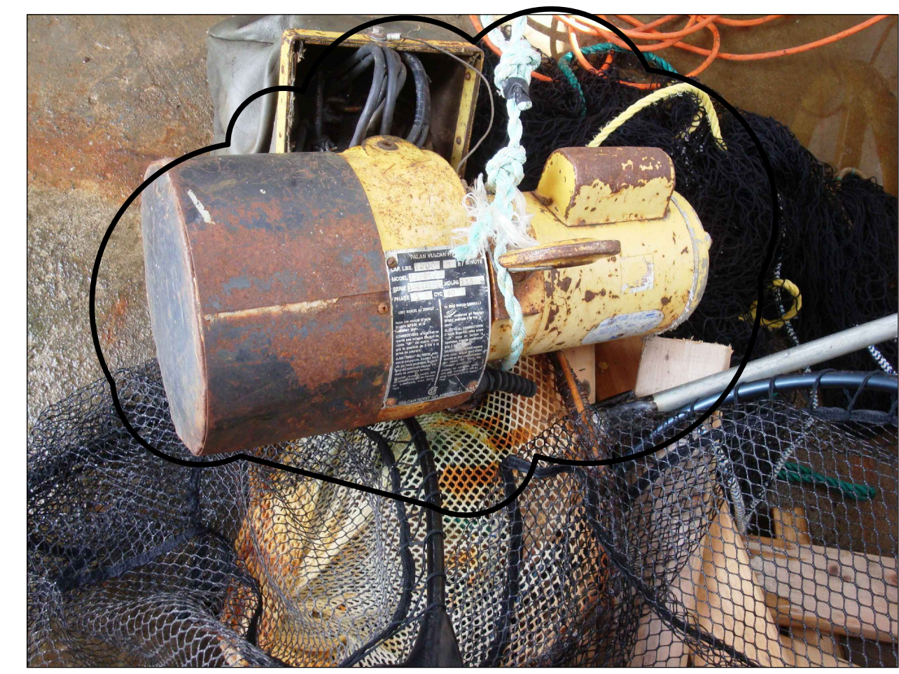
NOTE 10: REPLACE EXISTING VULCAN WIRE ROPE HOIST: SUPPLY TO THE OWNER, ONE (1) NEW VULCAN HOIST MODEL HOU2A07 -115AMP/1/60HZ-20- ONE TONNE WIRE ROPE HOIST COMPLETE WITH 20 HOUQZINC TREATED CHAIN, HOUAZINC-HOOK- 1F HOOK TREATMENT, HOUAACIDITY MOTOR TREATMENT, HOUATEFC MOTOR, HOUASYNTHETIC OIL, HOUANA30 CHAIN CONTAINER, LIFT, CABLE AND HOUAREMOT4 ONE (1) RECEIVER AND TWO (2) RADIO TRANSMITTERS AND WIRED CONTROLLER BACKUP
