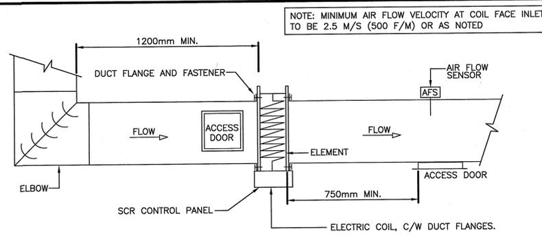
DUCT MOUNTED ELECTRICAL REHEAT COIL DETAIL
