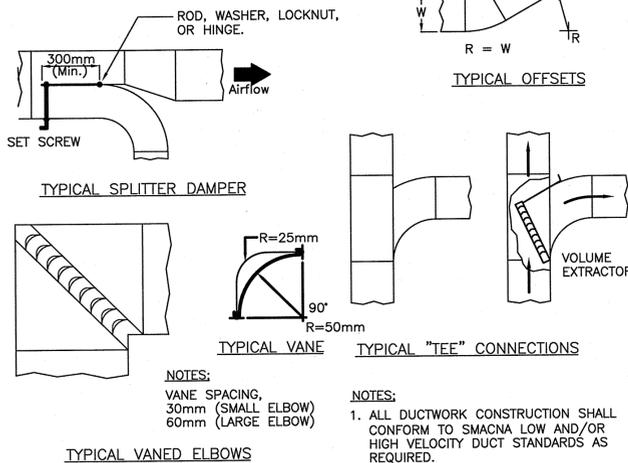
TYPICAL DUCT CONSTRUCTION DETAILS
