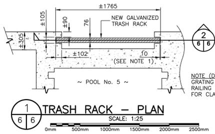
NOTE (DETAIL 1): GRATING AND RAILING OMITTED FOR CLARITY.
