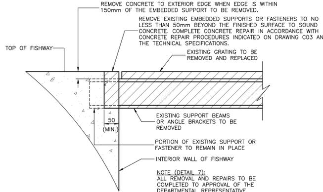
7 REMOVAL OF CONCRETE EMBEDDED SUPPORTS AND FASTENERS - TYPICAL
