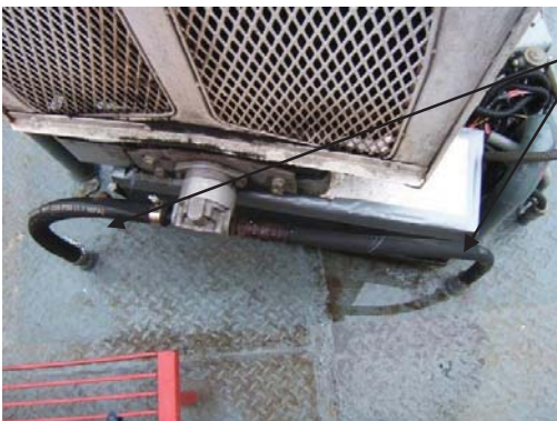
Current hose penetrations in scow deck.
