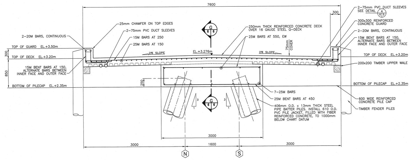
**FINGER WHARF CONCRETE DECK AT BATTER PILE CLUSTER DETAIL** (5/4/6)
