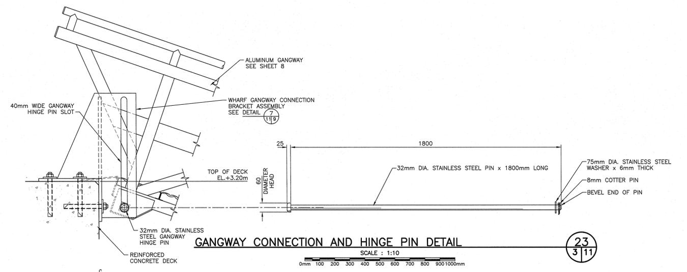
**GANGWAY CONNECTION AND HINGE PIN DETAIL**
