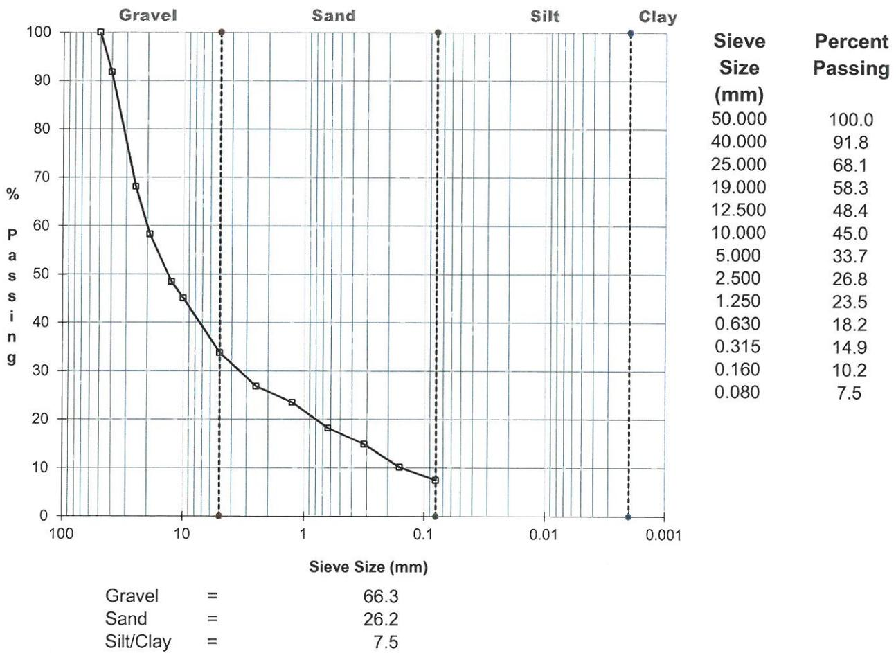
Sample Description: Gravel, some sand, trace silt, trace clay
