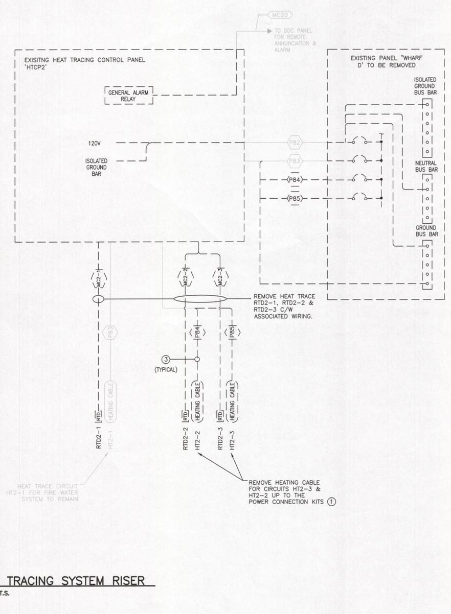
**EXISTING AND DEMOLITION HEAT TRACING SYSTEM RISER**
