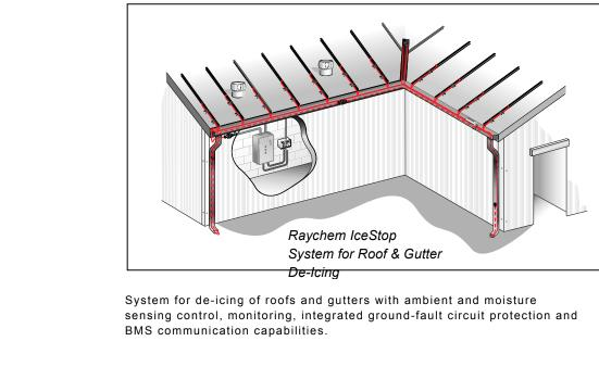
This specification describes an energy efficient de-icing system for roofs, gutters and downspouts, various attachment methods and control systems. Depending on the system design and size of application, one of the three control options listed should be selected.
