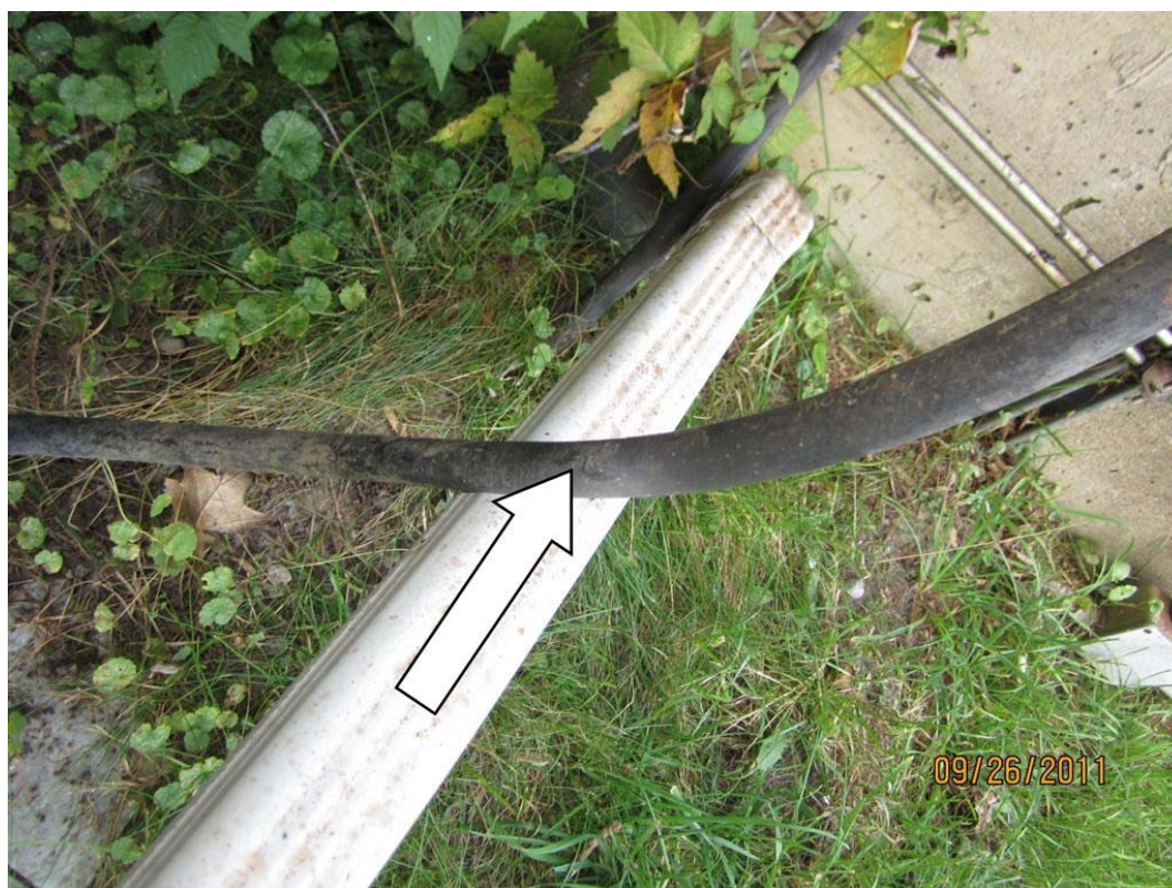
Photo M20: The west locking pin hydraulic cylinder blind end hose (arrow) is damaged.
