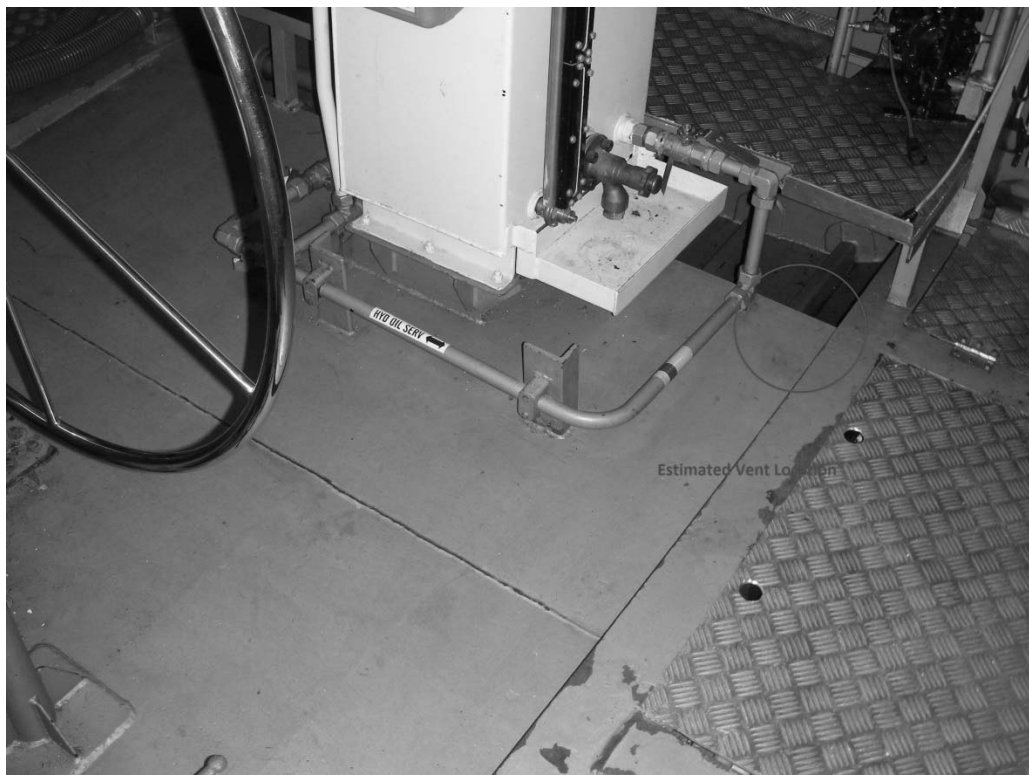
Figure H-02-2 Fuel Tank #9 Proposed Vent Location
