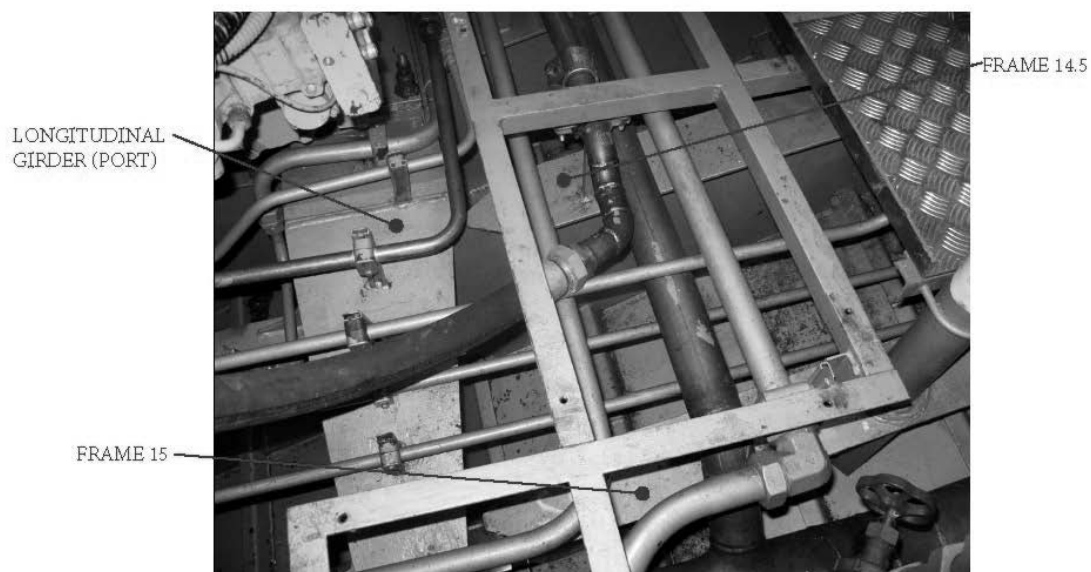
4. Main Engine Room - View of outboard (Port) engine support girder (looking aft).
