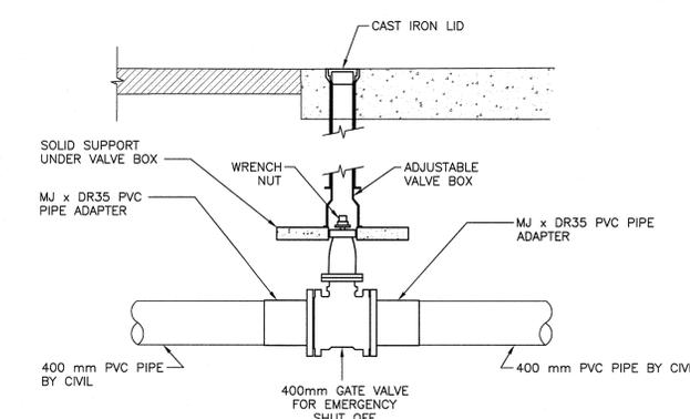
**EMERGENCY SHUT OFF VALVE DETAIL O.W.S.**
