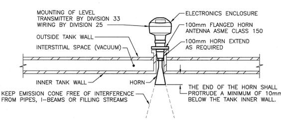
**RADAR LEVEL DETECTOR DETAIL**
