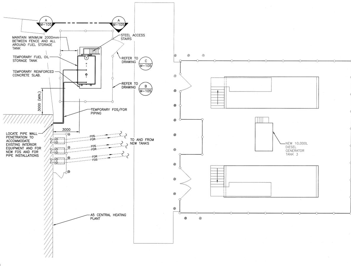
**PART PLAN - TEMPORARY FUEL OIL TANK ARRANGEMENT**
