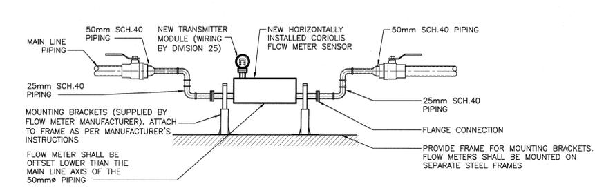
**FLOW SENSOR INSTALLATION DETAIL**
