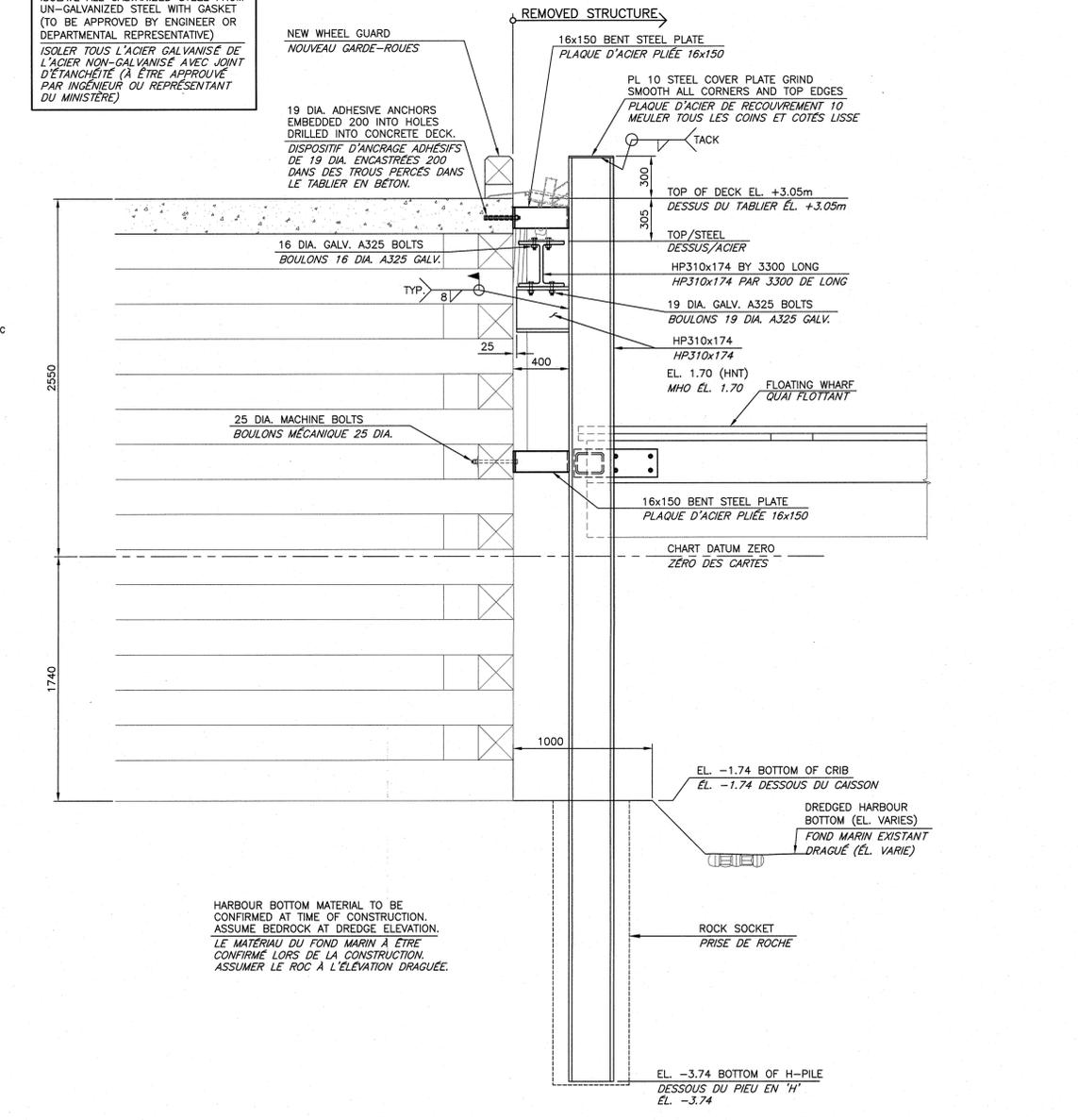
**SECTION AT FLOATING WHARF ANCHORAGE**
