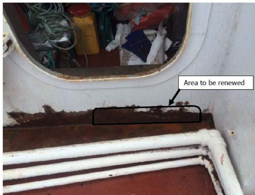
Photograph 2: Longitudinal bulkhead for SAR Locker
