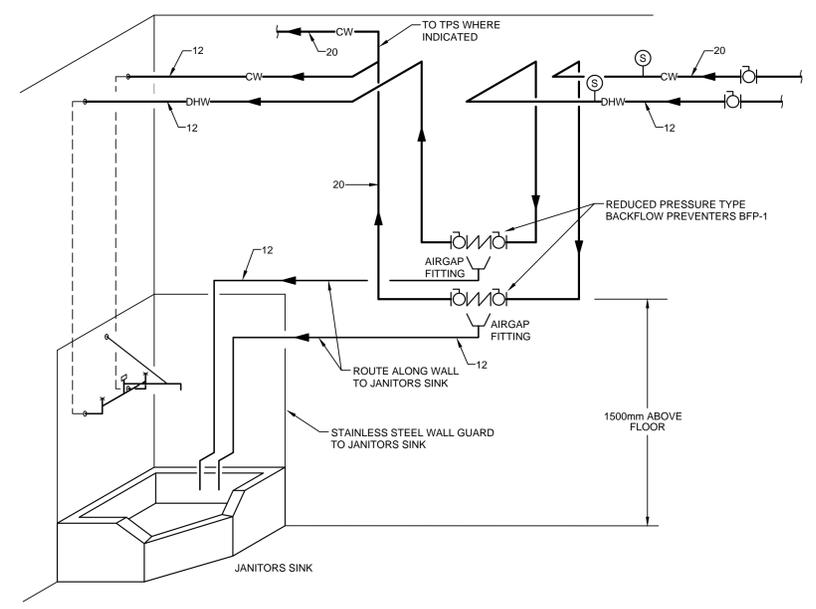
TYPICAL JANITOR'S SINK PIPING DETAIL
