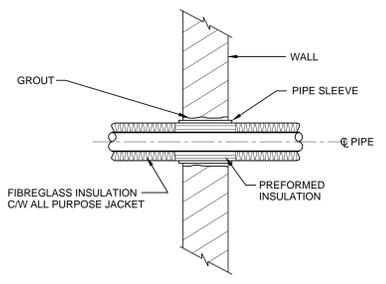
TYPICAL HOLE THRU BLOCK/TILE WALL
