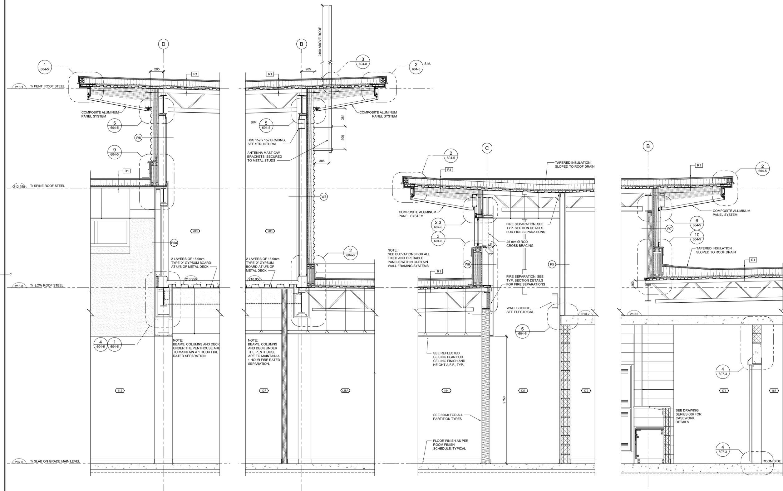
WALL SECTION-AT PENTHOUSE/ SPLINE JUNCTION C
