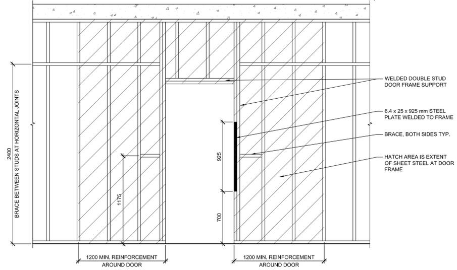
ELEVATION - SECURE (SR-2) WALL FRAMING 2
