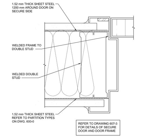
SECURE (SR-2) WALL/DOOR FRAME DETAIL 4
