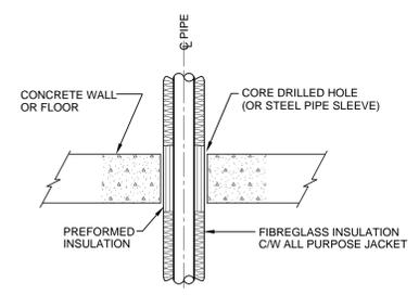
TYPICAL HOLE THRU CONCRETE WALL/FLOOR DETAIL
