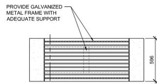
NOTE: PROVIDE CONCEALED FASTENERS THROUGH GALVANIZED METAL FRAME FOR SLAT SECUREMENT AT ANY END OR INTERMEDIATE FRAME MEMBER
