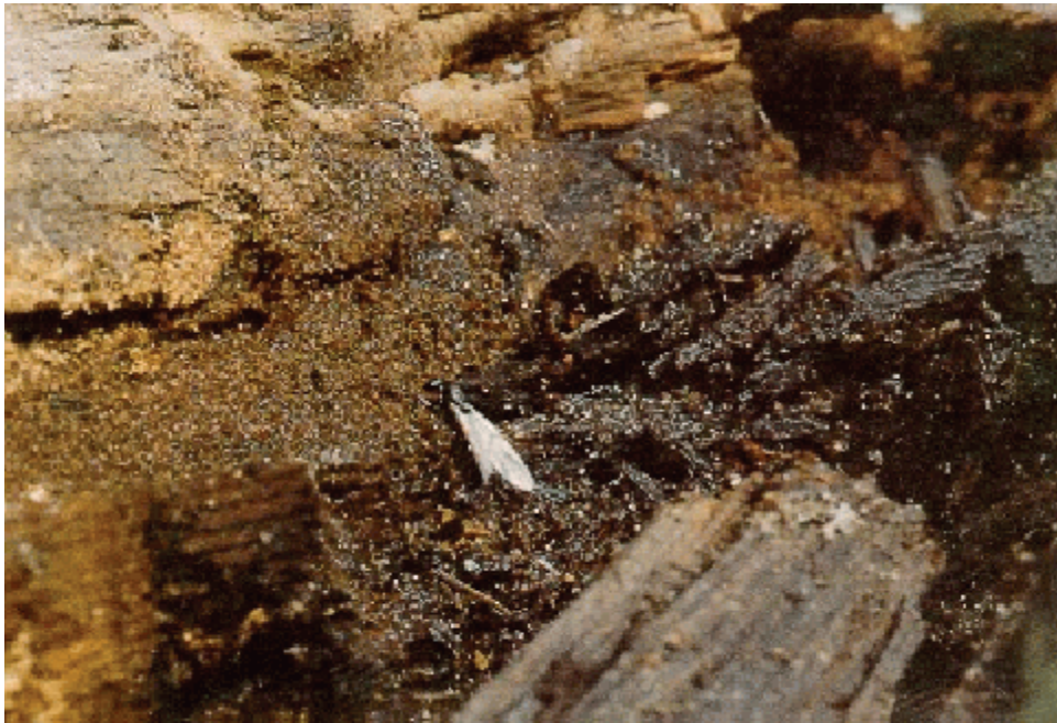
Figure 2.4.3(b) Very Severe Insect Damage in Wood
