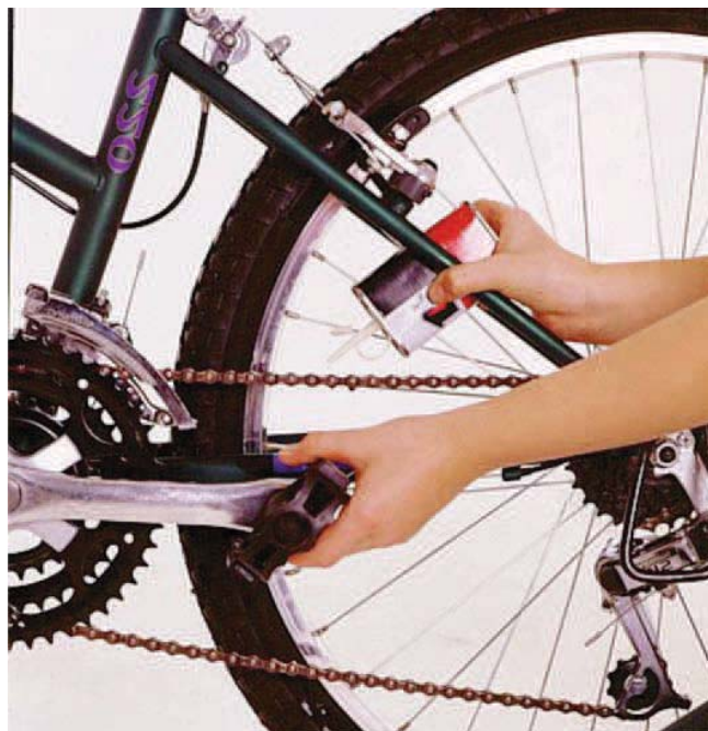
Figure 5 Lubricating the Chain
