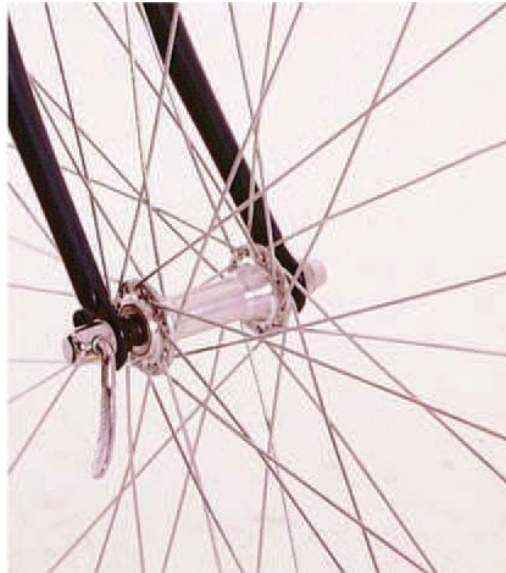
Figure 6 Quick Release Incorrect Position—Example 1
