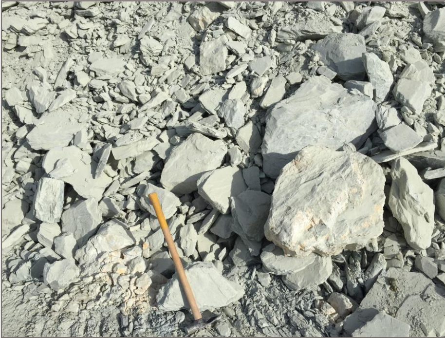
Photo 33: Typical excavation material at the base of the rock slopes within the Phyllite Rock Slope section. Observed lithology is a homogeneous carbonaceous phyllite unit, with minor interbedded quartz veining, oriented parallel to and perpendicular to phyllite foliation. Photo taken at Station 124+300.
