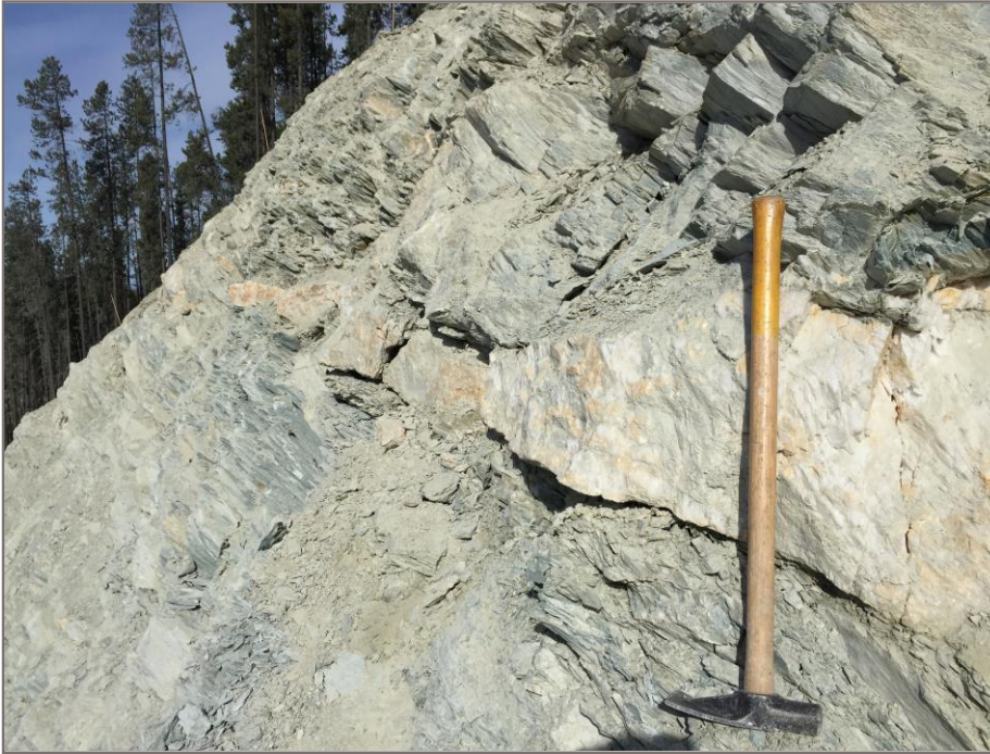
Photo 35: Quartz vein (30-40cm width) interbedded between the carbonaceous phyllite unit, at Station 124+550. Quartz veining was visually approximated to represent 5% of the exposed rock slope, with the homogeneous phyllite unit representing the remaining 95%.
