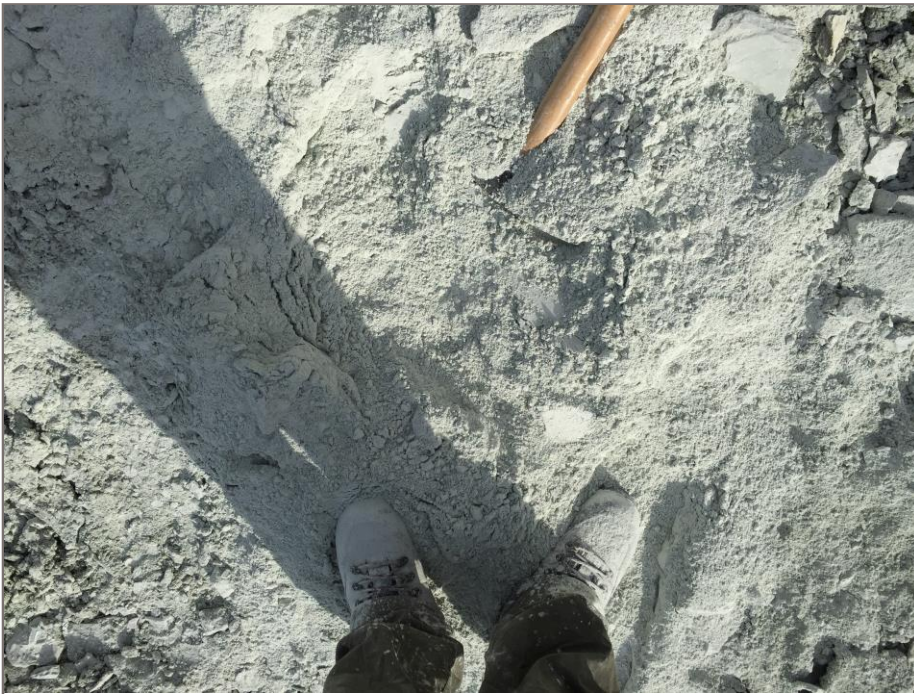
Photo 34: Phyllite material disintegrates into a very fine grained, low density powder during excavation.
