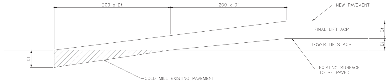
TYPICAL MILLED TIE-IN TO EXISTING ASPHALT NTS
