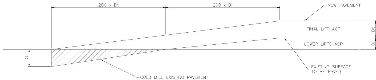
TYPICAL MILLED TIE-IN TO EXISTING ASPHALT NTS
