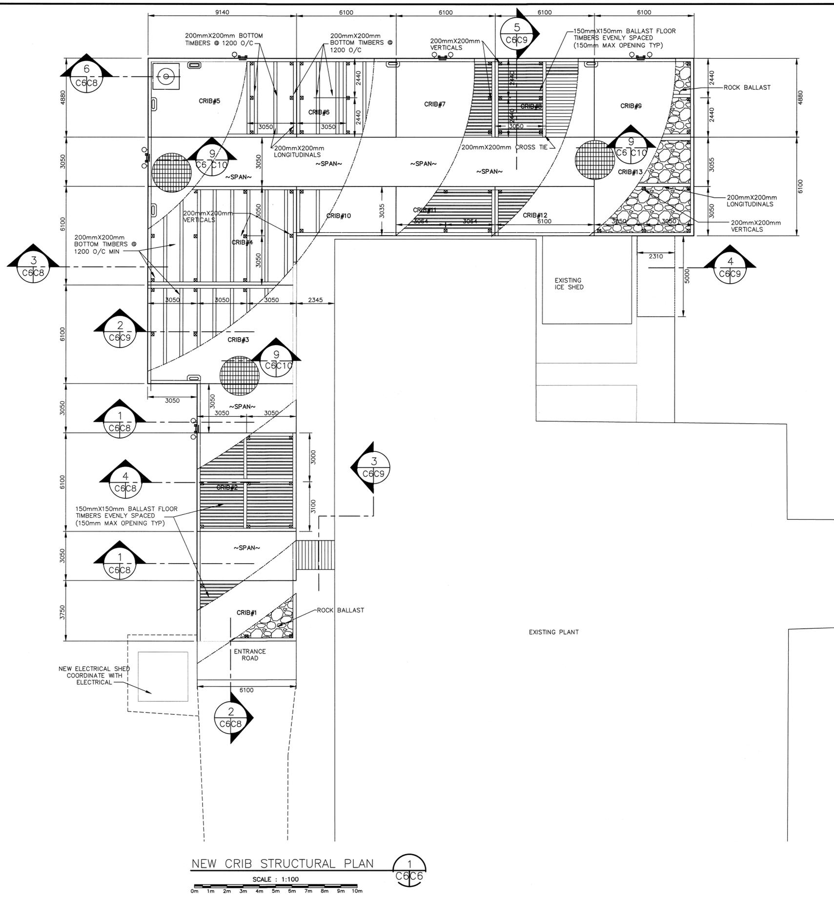
NEW CRIB STRUCTURAL PLAN
