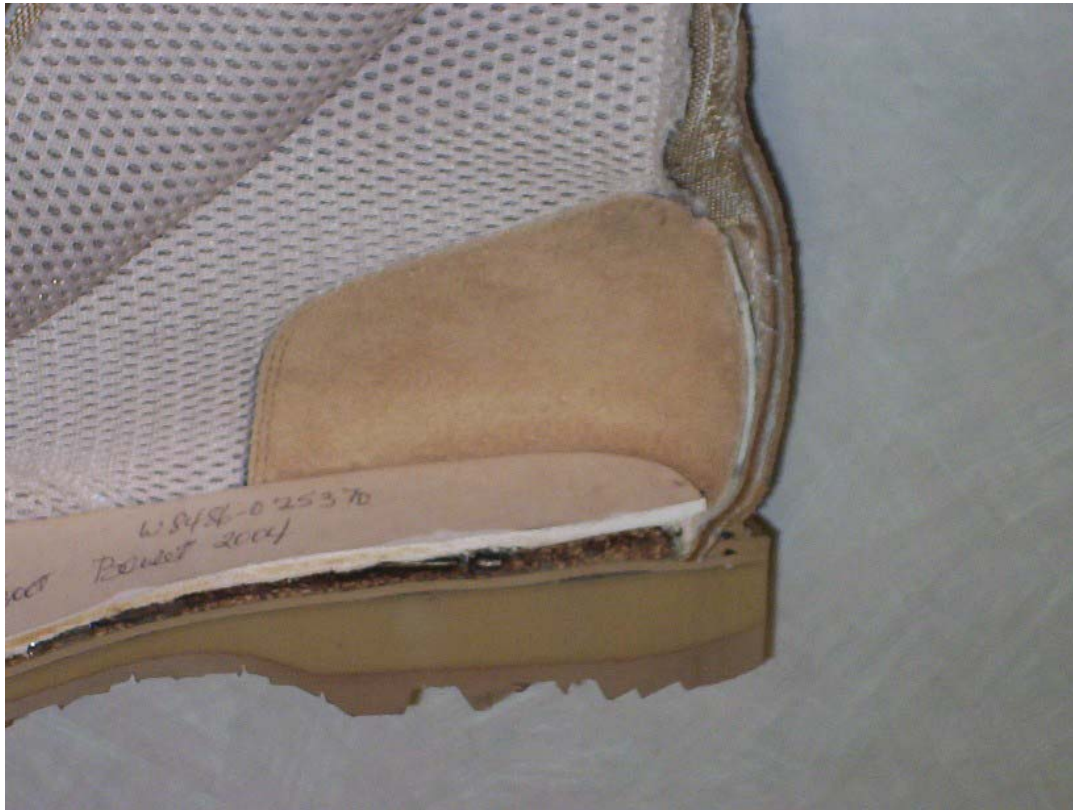
Figure 7: Heel/counter area to show counter pocket/lining assembly. Note 1 - Lining type to be in accordance with the specification Note 2 - Outsole 601-3 has a heel breast
