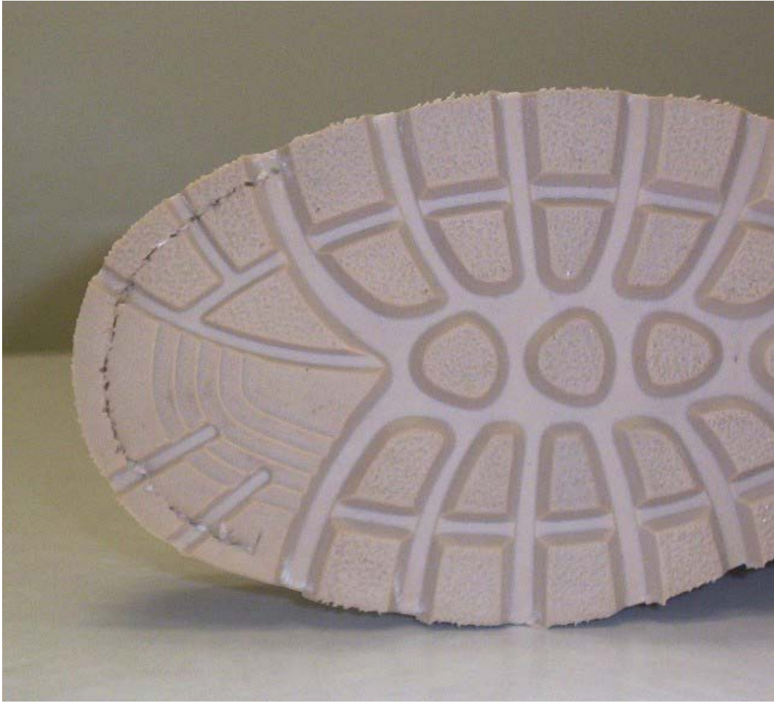
Figure 8: Close-up view of safety stitch in toe area.
