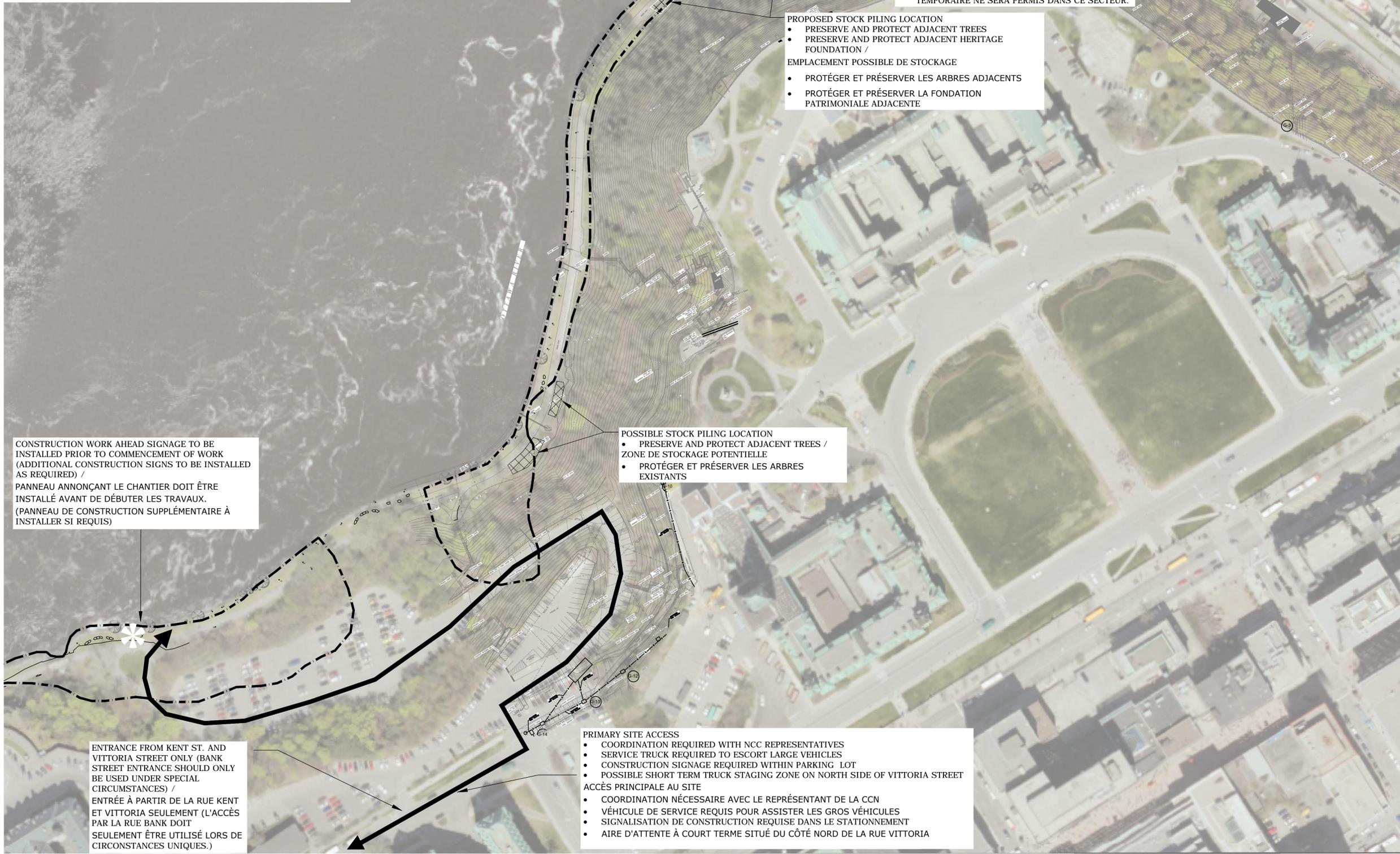
CONSTRUCTION WORK AHEAD SIGNAGE TO BE INSTALLED PRIOR TO COMMENCEMENT OF WORK (ADDITIONAL CONSTRUCTION SIGNS TO BE INSTALLED AS REQUIRED) / PANNEAU ANNONÇANT LE CHANTIER DOIT ÊTRE INSTALLÉ AVANT DE DÉBUTER LES TRAVAUX. (PANNEAU DE CONSTRUCTION SUPPLÉMENTAIRE À INSTALLER SI REQUIS)
