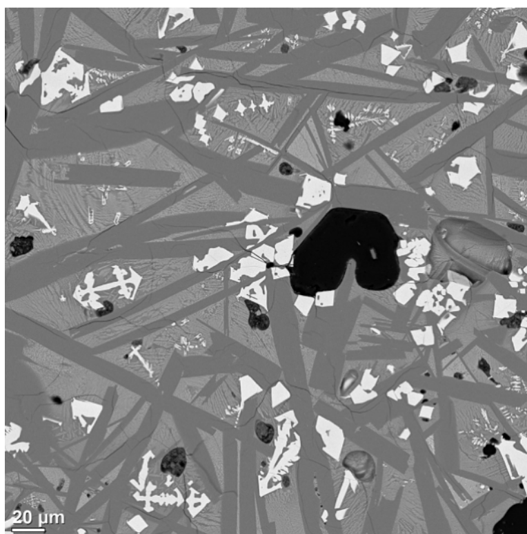
Figure 14: Higher magnification image of Fragment 20 from Figure 13, consisting of relatively coarse anorthite blades (medium grey), skeletal and cruciform Fe-oxide (white) in a devitrified glassy matrix that exhibits a feathered texture.
