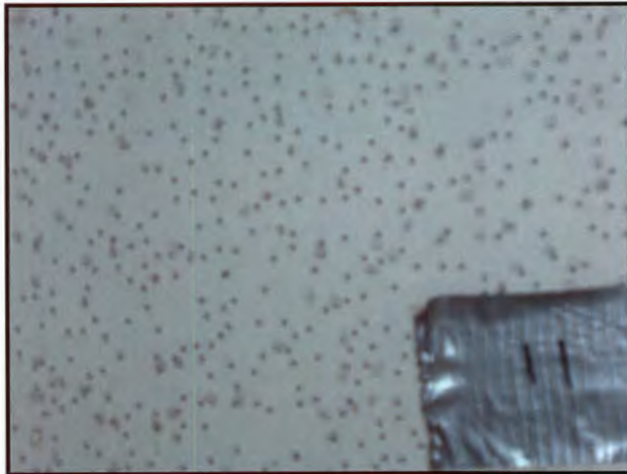
Photograph 11: Sample 124-B7-11, 2' x 2', Small and Medium Pinholes / Ceiling Tile
