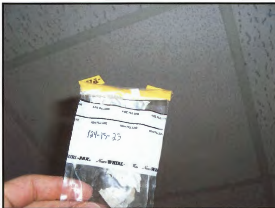
Photograph 22: Sample 124-15-23, 2' x 2', Small and Medium Pinholes / Ceiling Tile
