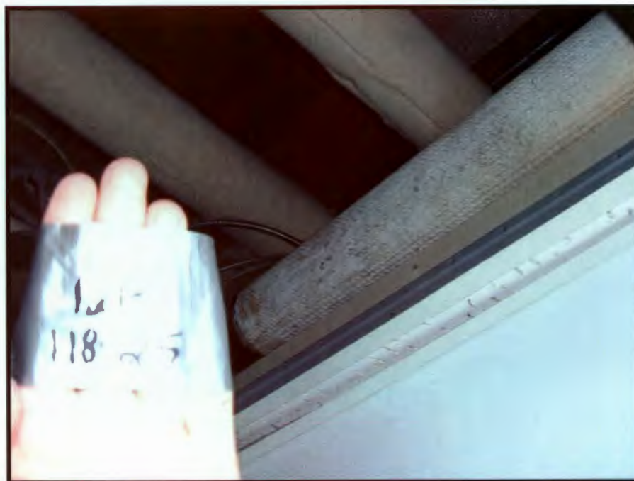
Photograph 24: Sample 124-118-25 / Cement Pipe
