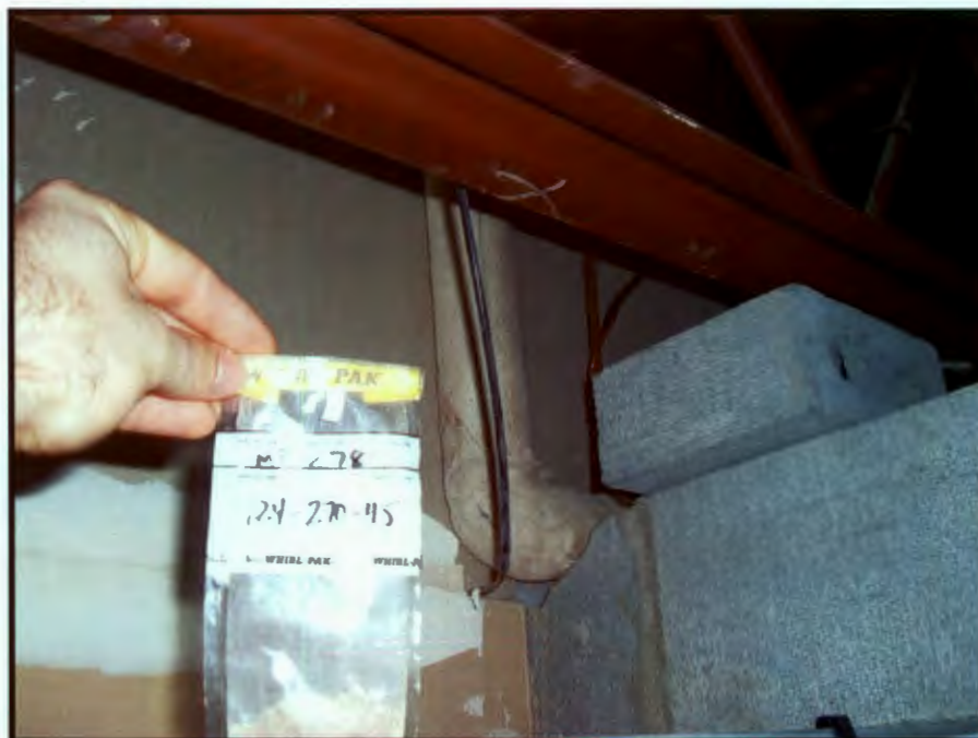
Photograph 44: Sample 124-270-45 / Mudding on Pipe Elbow
