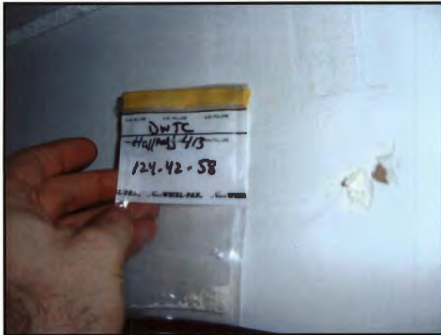
Photograph 57: Sample 124-42-58, above Ceiling Tile / Drywall Joint Compound
