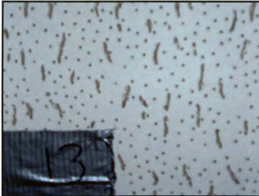
Photograph 13: Sample 124-B7-13, 2' x 4', Medium Random Pinholes with Fissures / Ceiling Tile
