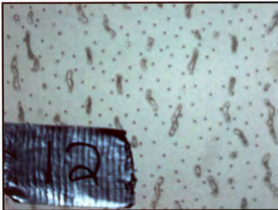
Photograph 12: Sample 124-B7-12, 2' x 2', Small Random Pinholes with Deep Fissures / Ceiling Tile
