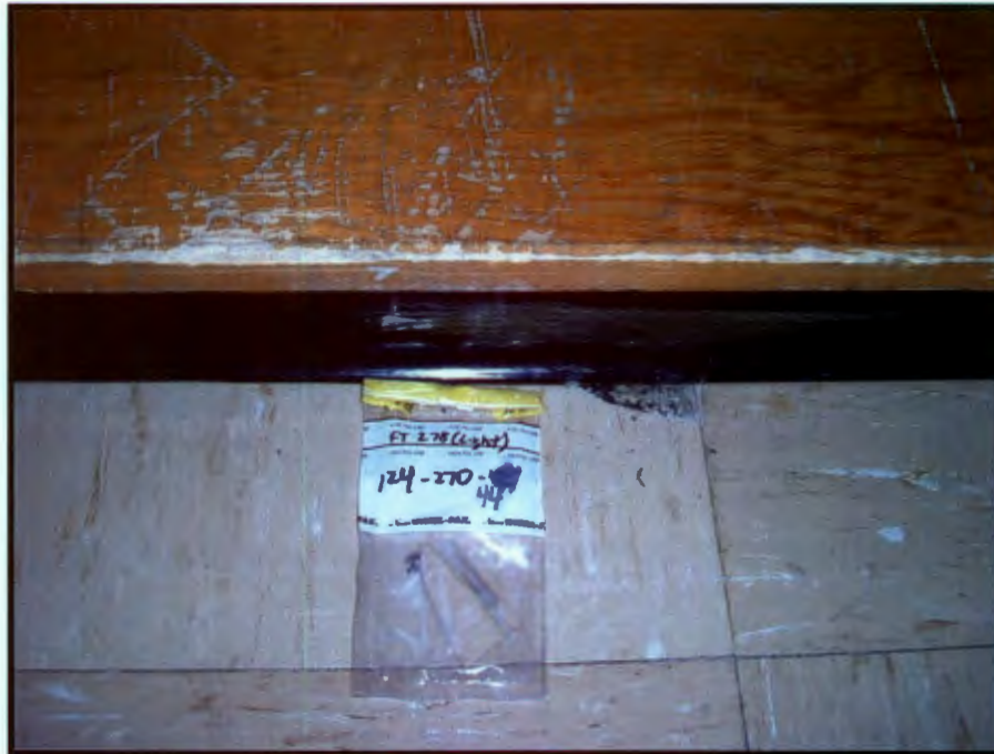
Photograph 43: Sample 124-270-44, 12"x 12", Light Beige with White and Brown Streaks / Floor Tile
