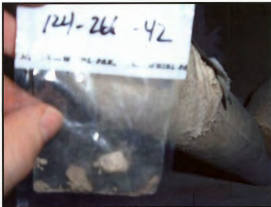
Photograph 41: Sample 124-266-42 / Mudding on Pipe Elbow
