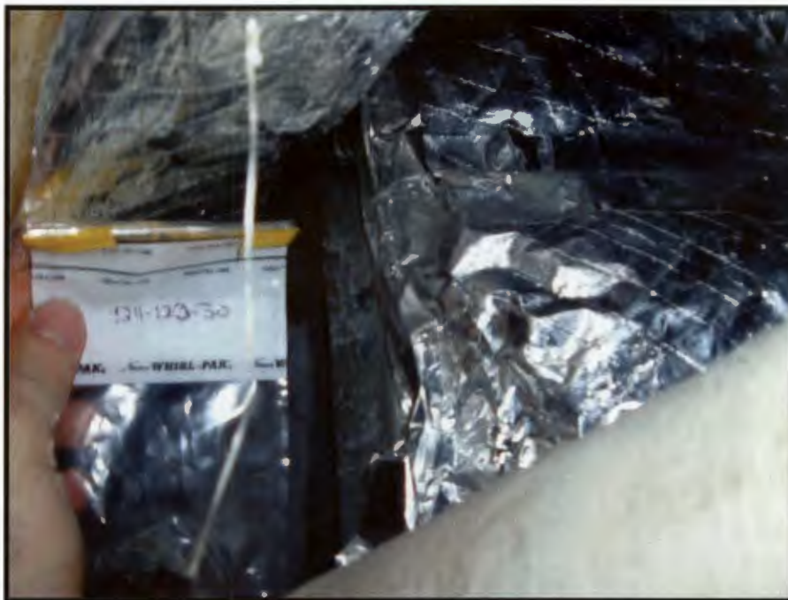
Photograph 29: Sample 124-120-30, First Floor / Duct Joint Mastic
