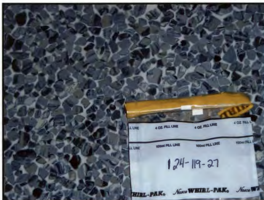
Photograph 26: Sample 124-119-27, Blue, Gray, and Beige Aggregate / Sheet Flooring
