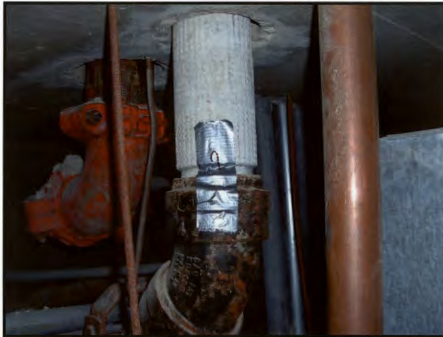
Photograph 9: Sample 124-B1-9 / Cement Pipe
