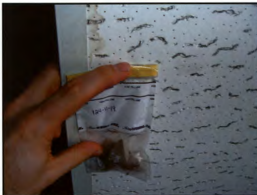
Photograph 18: Sample 124-11-19, 2' x 2', Small Random Pinholes with Deep Fissures / Ceiling Tile
