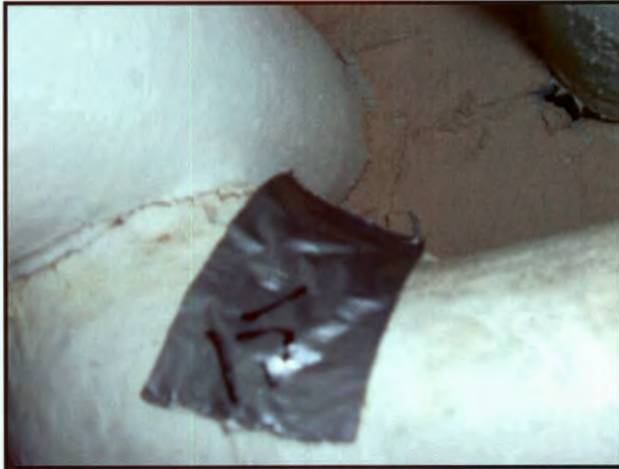
Photograph 15: Sample 124-B5-15, Hot Water Supply Line (Smaller) / Mudding on Pipe Elbow
