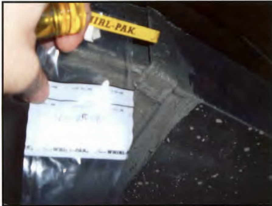
Photograph 45: Sample 124-25-46, above Ceiling Tile / Duct Joint Mastic
