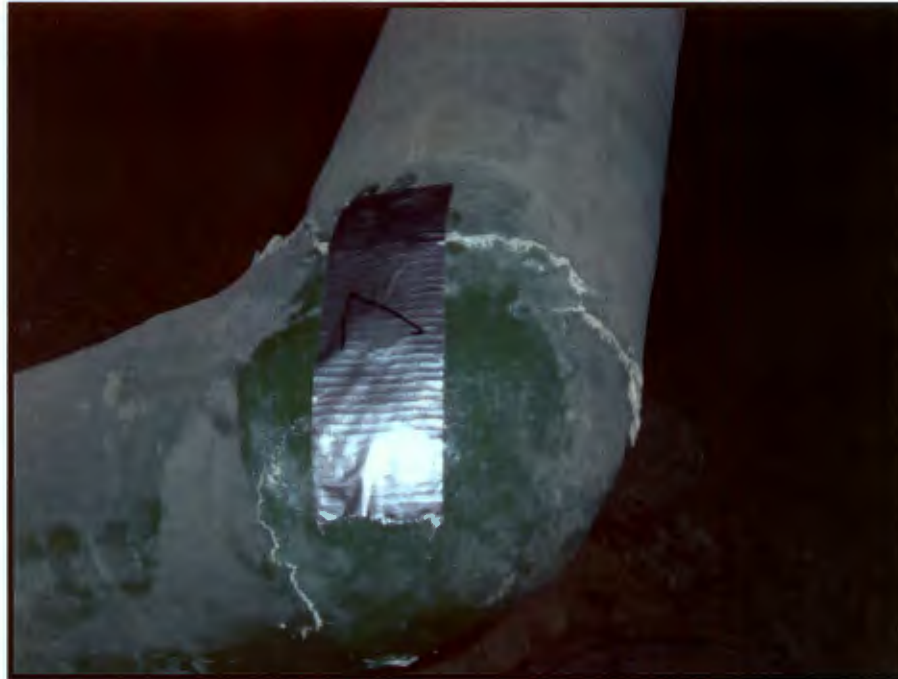
Photograph 7: Sample 124-B1-7, Green Pipe, High Pressure Condensate / Mudding on Pipe Elbow
