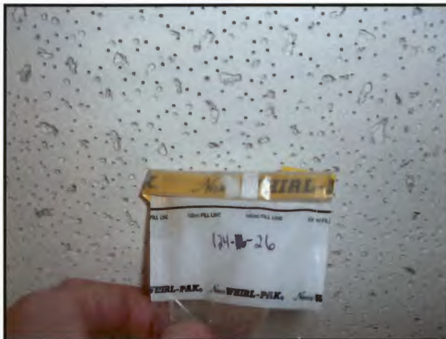
Photograph 25: Sample 124-116-26, 2' x 2', Small and Medium Pinholes with Small Fissures / Ceiling Tile
