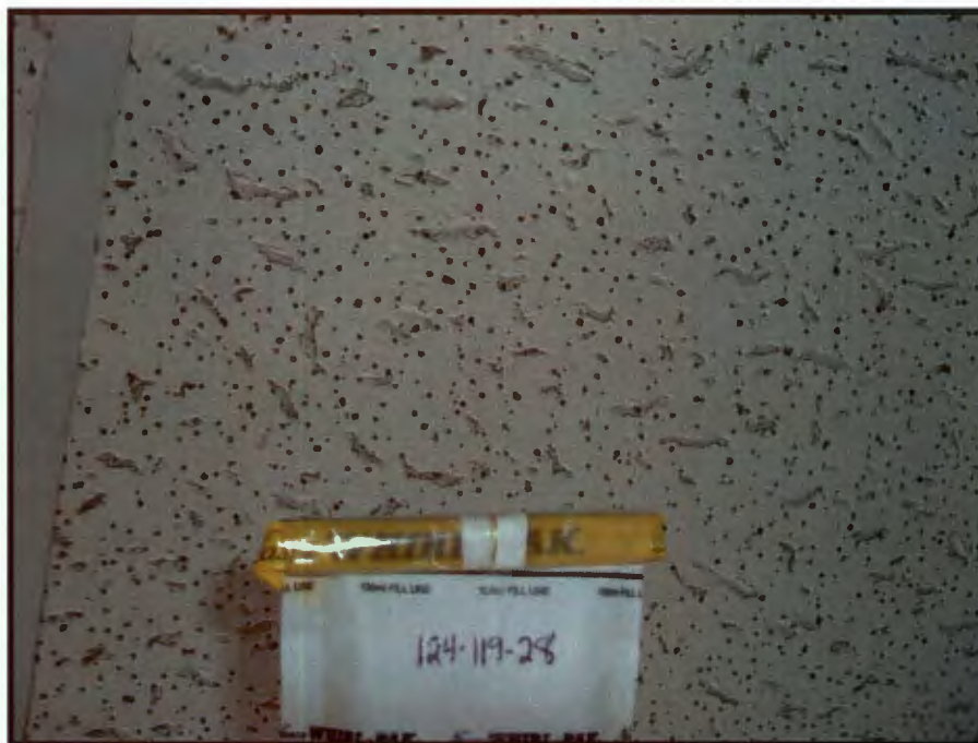
Photograph 27: Sample 124-119-28, 2' x 2', Varied-Sized Pinholes with Long Fissures / Ceiling Tile
