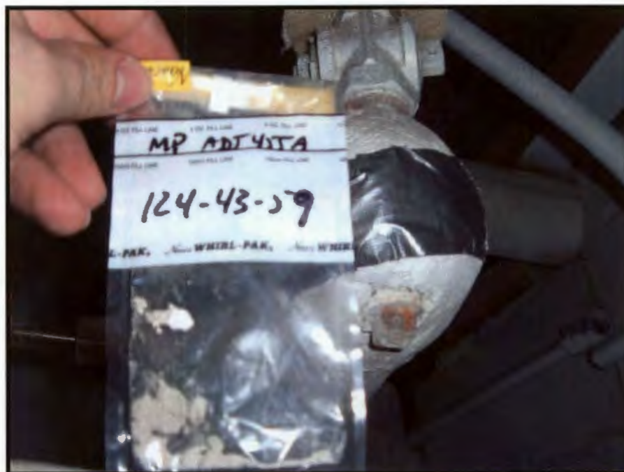
Photograph 58: Sample 124-43-59, Adjacent to Room 455A / Mudding on Pipe Elbow
