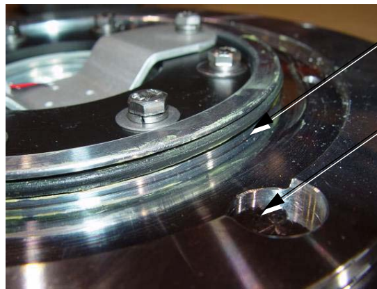
Figure 11: Replacing Cover/Inner Cover O-ring Seal
