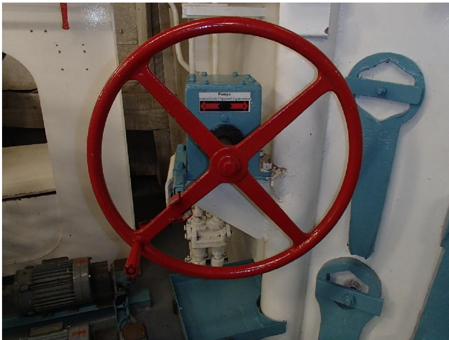
Photo no. 22 : Direct Emergency Helm Pump – Barre directe
