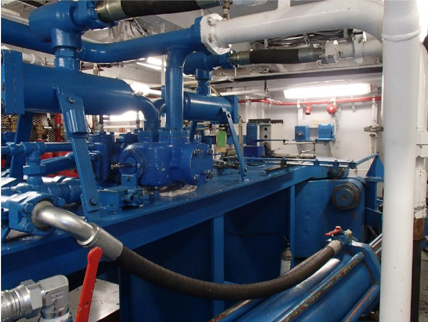
Photo no. 32 : Amundsen 4-Way Valve – Soupape 4 voies
