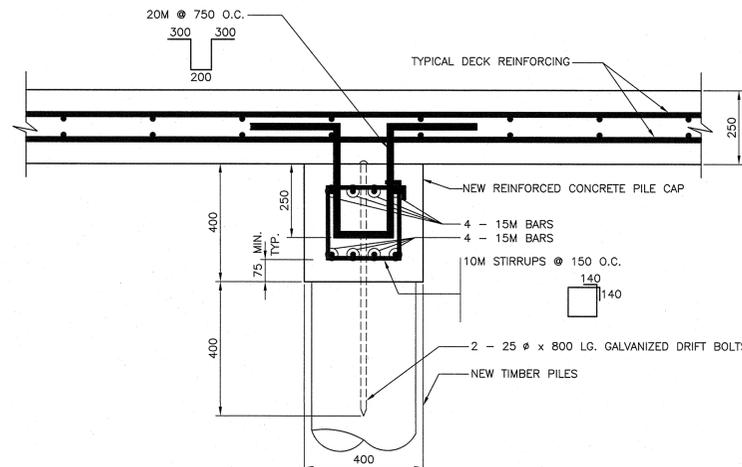
**NEW CONCRETE DECK SECTION AT PILE CAPS**
