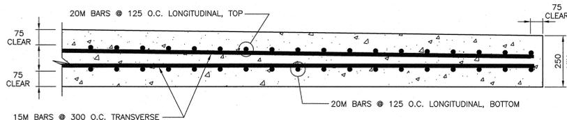
**SECTION THROUGH DECK SHOWING REINFORCEMENT**
