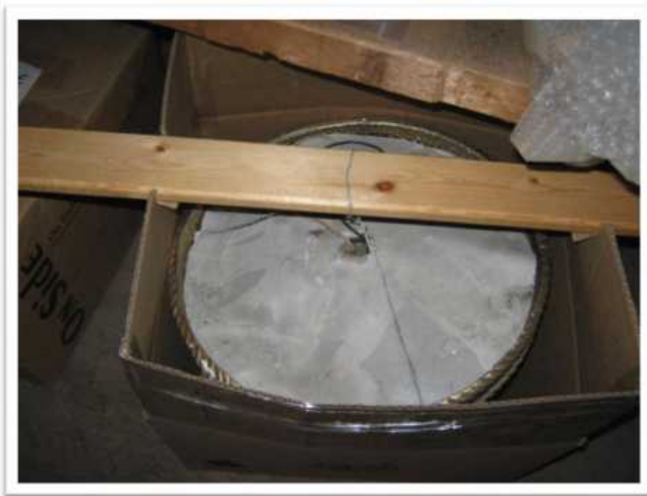
Photo 18: Light heat shields on light fixtures stored in the attic are suspected to contain asbestos.
