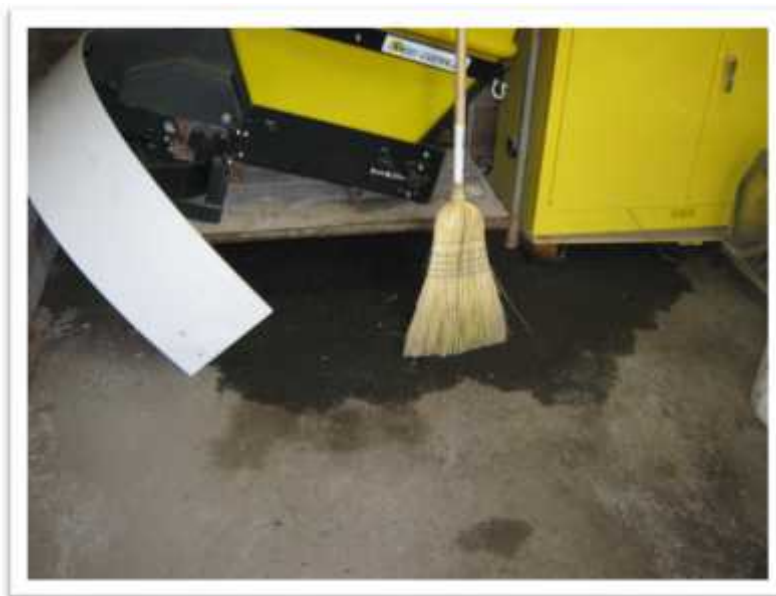
Photo 4: Typical example of a minor fuel spill on the concrete floor slab (which contains silica). In general, these spills appear to have been cleaned with adsorbent materials.
