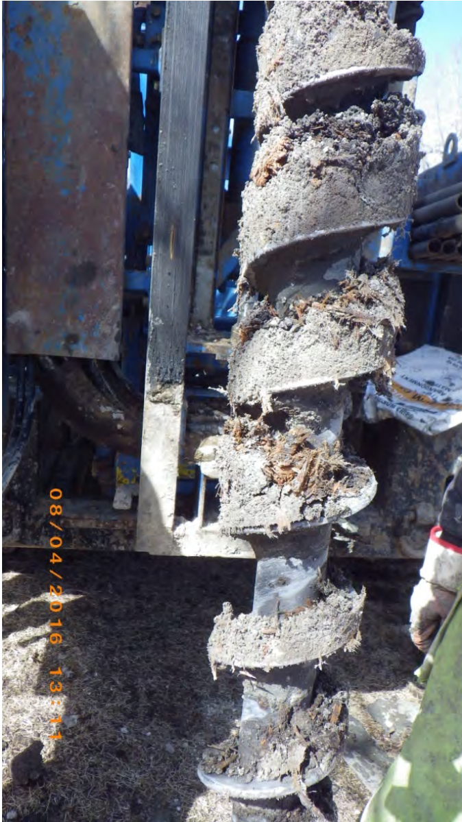
Figure 7. Wood fibres and sand identified in drill KGS Test 01 at approximately 2.5m – 3m depth.
