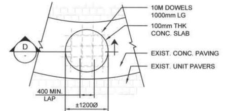
SECTION 3 CONCRETE INFILL DETAIL SCALE: 1:50
