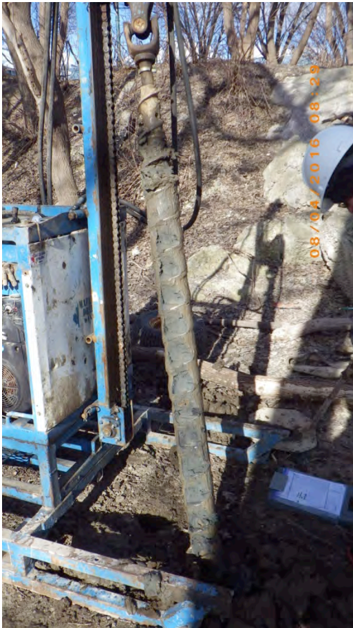
Figure 6. Examining soils from drill at 30cm increments for top 2m+.
