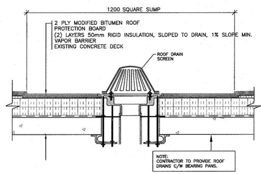
TYPICAL ROOF DRAIN DETAIL
