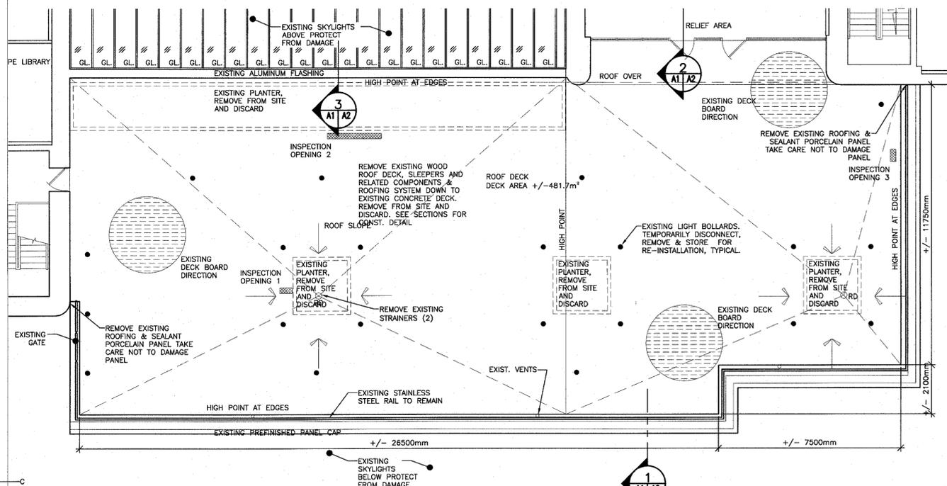
ROOF DECK - EXISTING DEMOLITION PLAN
