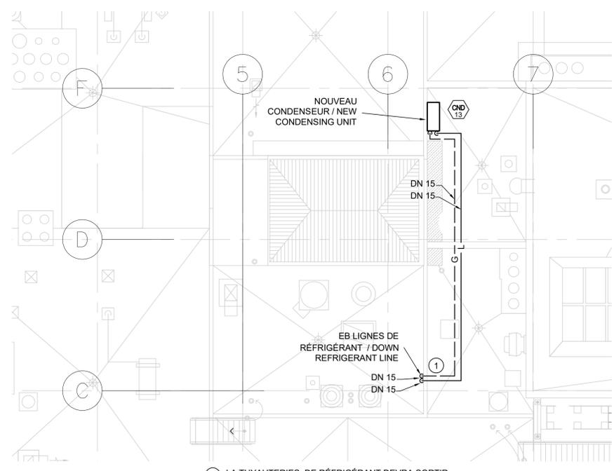
1 LA TUYAUTERIES DE RÉFRIGÉRANT DEVRA SORTIR À L'EXTÉRIEUR SUR LE CÔTÉ DE L'APPENTIS ET ÊTRE SOUTENIR SUR LE MUR EN REVÊTEMENT MÉTALLIQUE. REFRIGERANT LINES HAVE TO EXIT TO THE OUTSIDE THROUGH THE SIDE OF THE PENTHOUSE. THE REFRIGERANT LINES MUST BE ATTACHED ON THE METALIC SHEATING WALLS.
