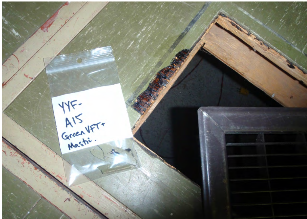
Photograph 31: Asbestos-containing green vinyl floor tiles ( Sample A15 ).
