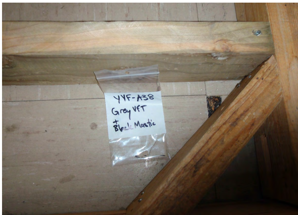
Photograph 38: Asbestos-containing grey vinyl floor tile ( Sample A38 ).
