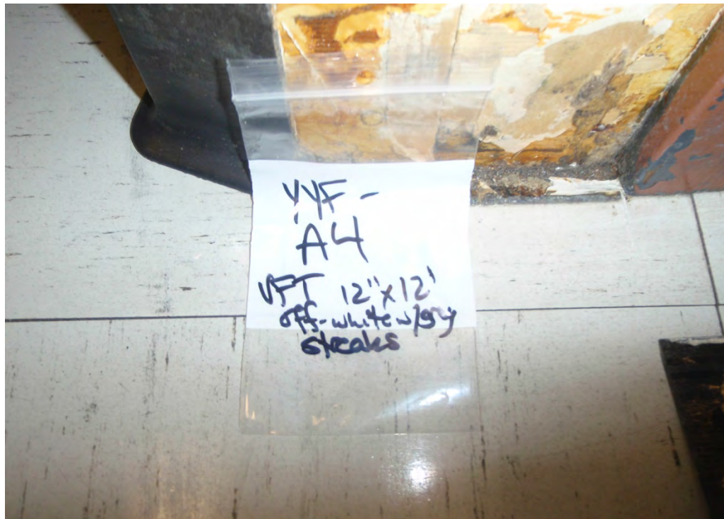
Photograph 29: Asbestos-containing light grey (off-white with grey streaks) vinyl floor tiles in Room 125 (Sample A4).
