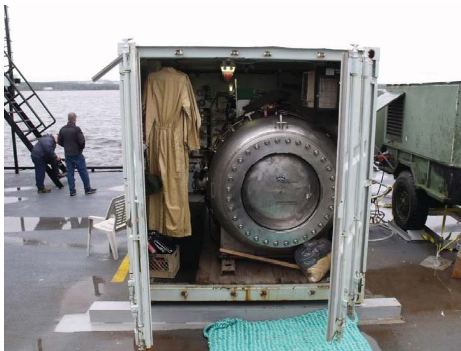
Figure 2: End view of the recompression chamber section of the Existing CDS RCC
