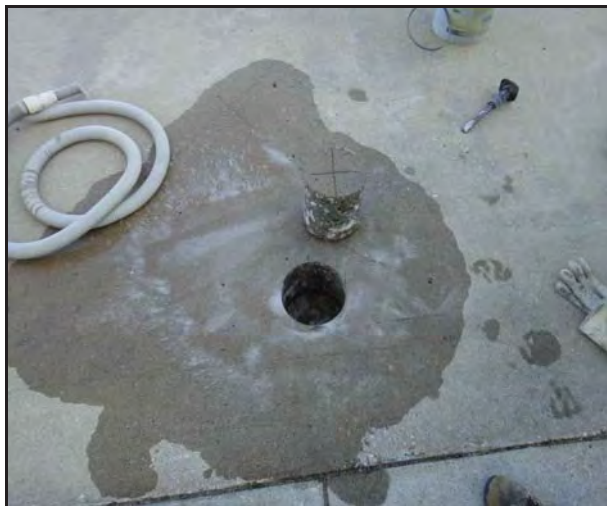
Photo 18 - Concrete core from test hole PA-10 located north of the RCMP Hangar.
