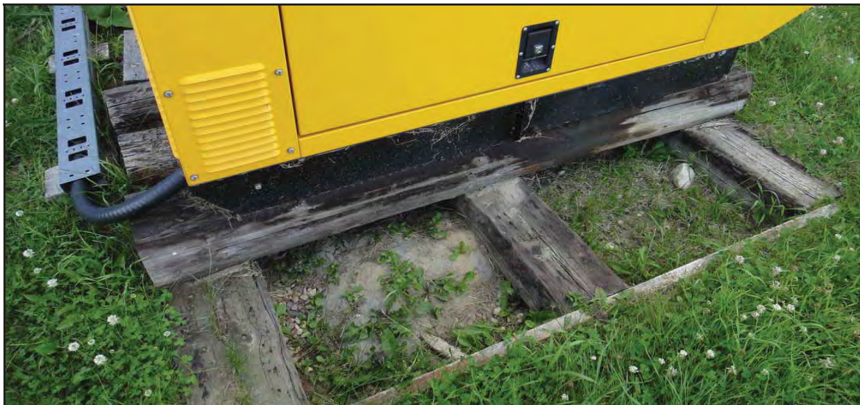
Photo 09 - Stained timber cribbing and discoloured soil on the east side of the diesel generator.
