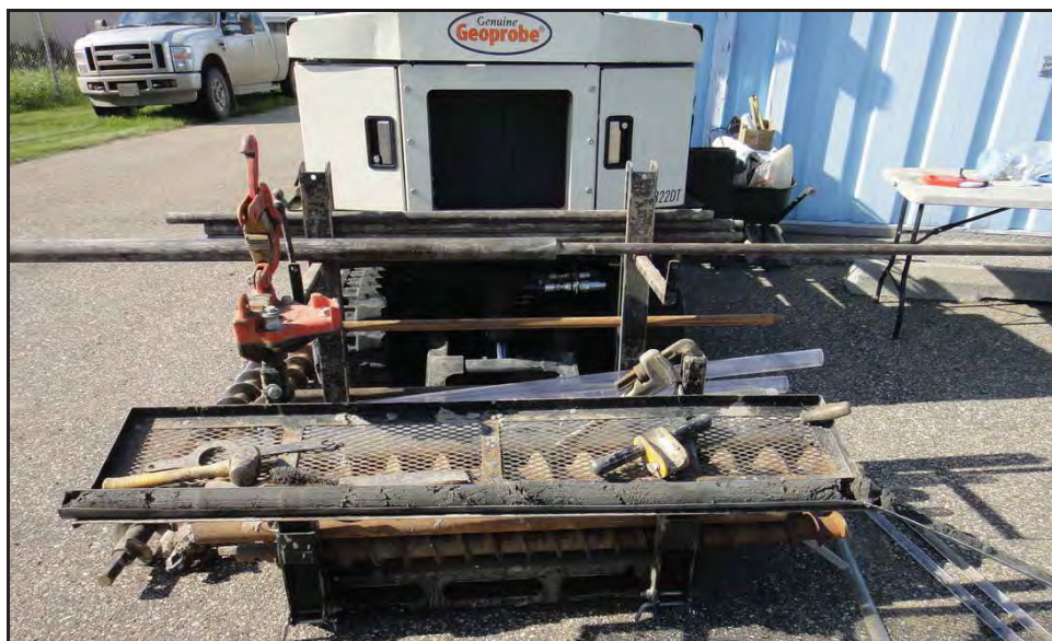
Photo 19 - Drill core tube extractor equipment and soil core ready for sampling.
