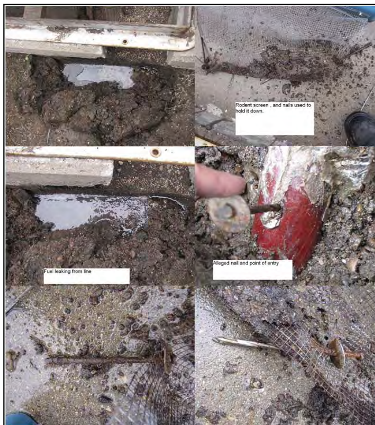
Plate 02 - Photographs taken from the 2010 Cantest Solutions Inc. - Leak Detection Report showing the nail puncture and leaking fuel line.
