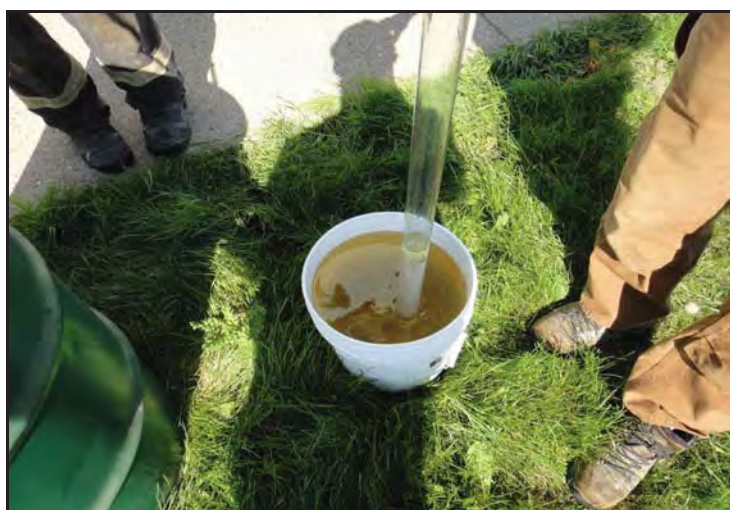
Photo 22 - Disposal of LNAPL into pail for transfer and storage in an on-site 220 litre drum.
