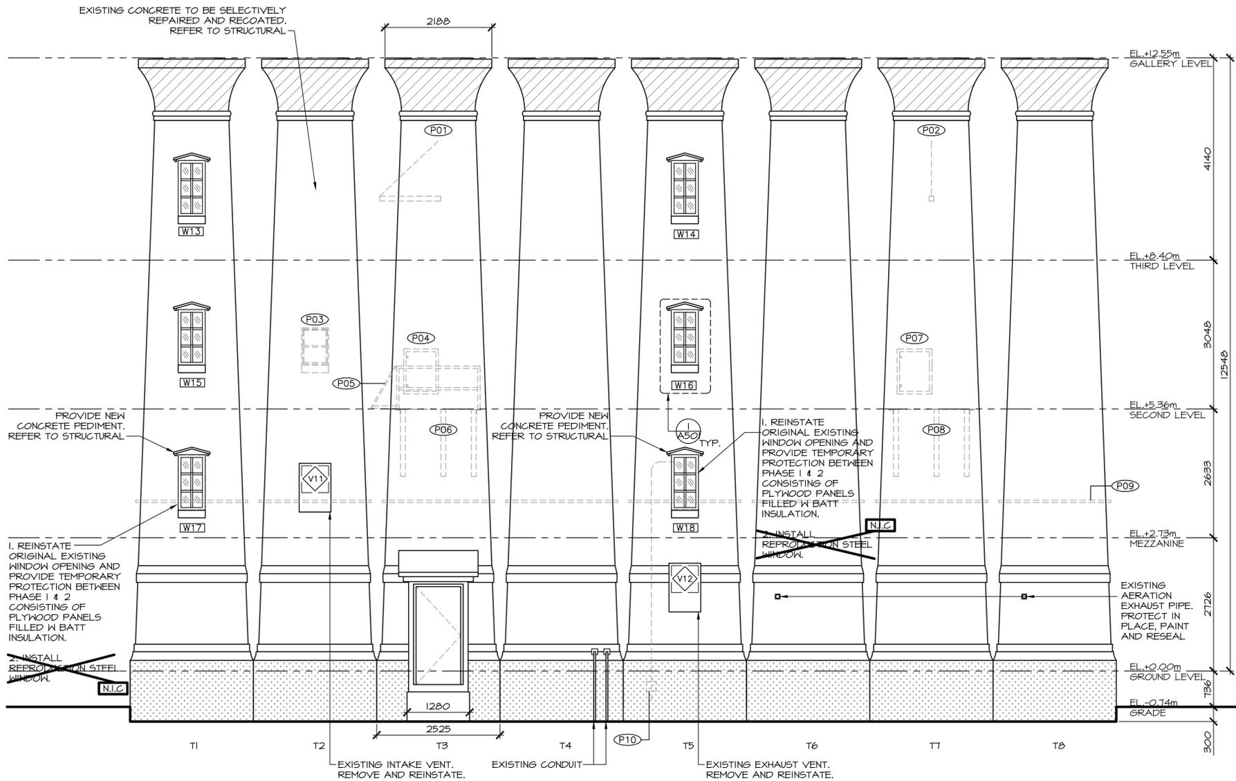
**TOWER EXTERIOR PEELLED ELEVATION**
