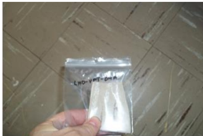
Photograph 4: [Lighthouse Keeper's Dwelling] Asbestos-containing 9"x9" pink vinyl floor tiles (Sample set LHD-VFT-4).
