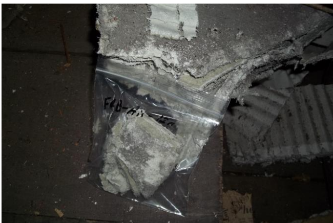
Photograph 5: [Fog Alarm Building] Asbestos-containing Air Cell pipe insulation debris observed in the attic (Sample set FAB-AIR-12).
