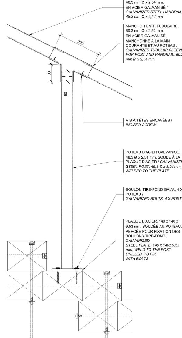
4 DÉTAIL MAIN-COURANTE / HANDRAIL DETAIL
