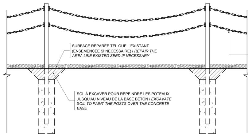
6 DÉTAIL CLÔTURE EXISTANTE À RESTAURER OU CLÔTURE TYPE CHAINETTE / EXISTING FENCE TO RESTORE OR FENCE WITH CHAIN DETAIL
