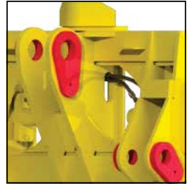
Machine pin-on hook-up of Quik Key Coupler.
