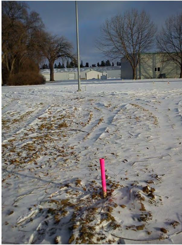
Photo 3 - Standpipe piezometer installed in Testhole TH 04
