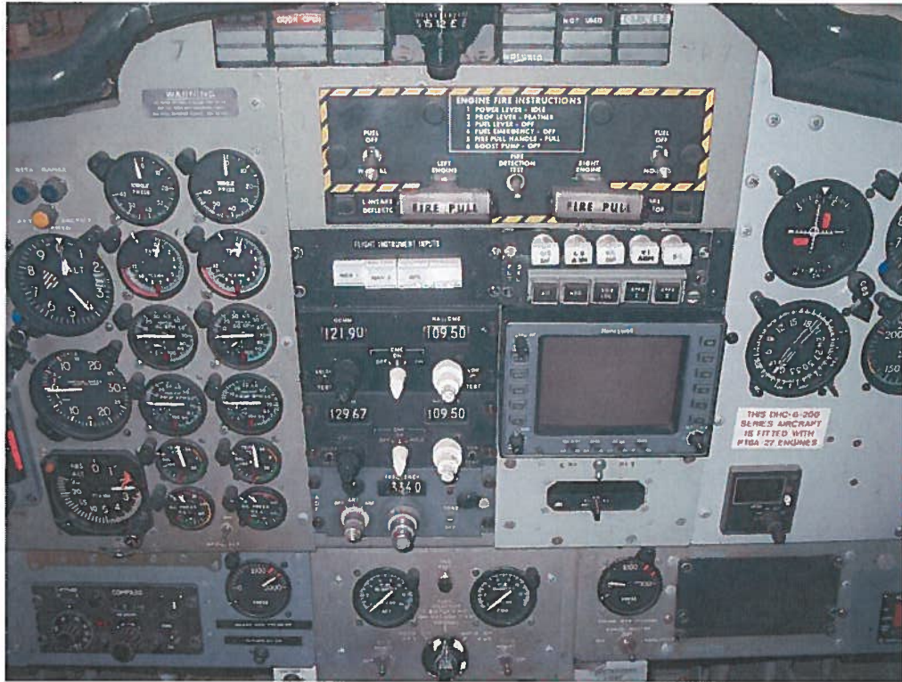
Figure B-2 Centre Instrument Panel
