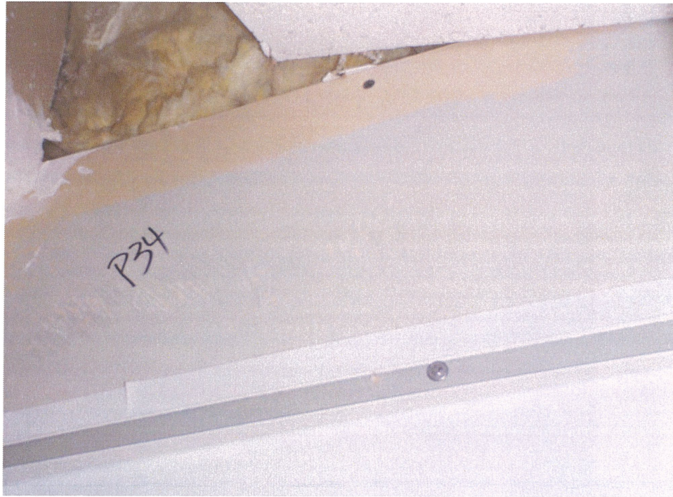
Photograph 81: Lead-based grey primer paint on wall in ceiling space of Room 142 ( Sample P34 ).
