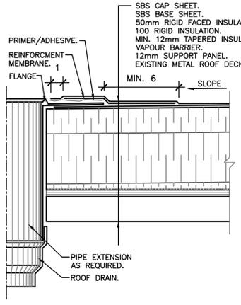
8 ROOF DRAIN DETAIL
