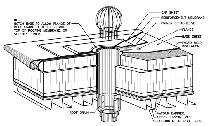
9 ROOF DRAIN DETAIL
