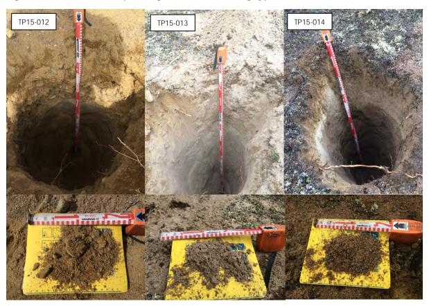
Figure 17: Photos of test pits dug at GD-28 showing typical material encountered
