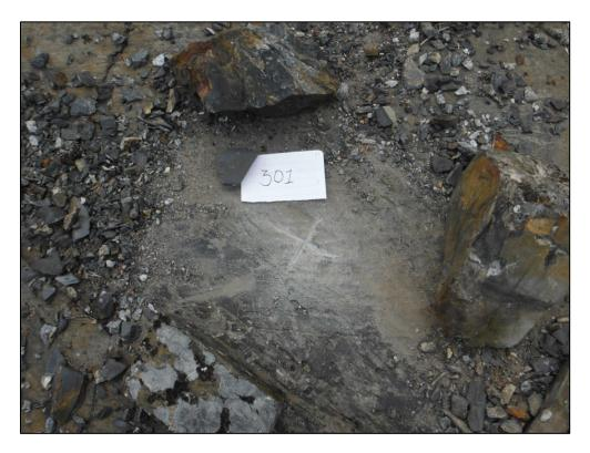
Photo 1: Placed survey control points
