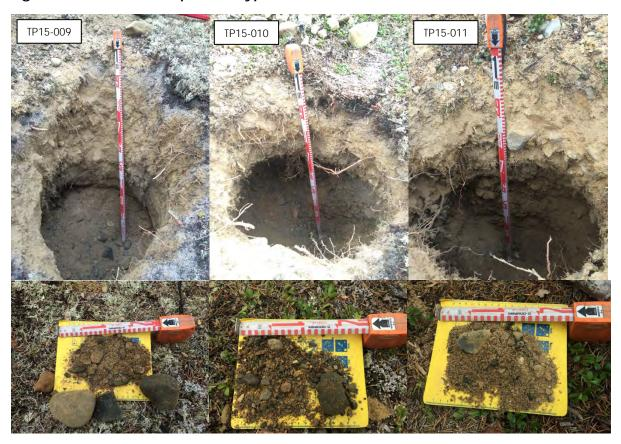
Figure 20: Photos of test pits and typical sub surface materials at GD-11.
