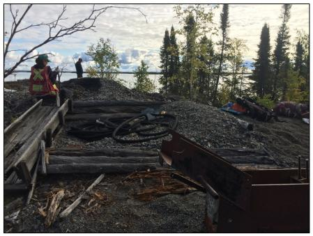
Photo 11: Wooden sluice present at the Treacy mine site.
