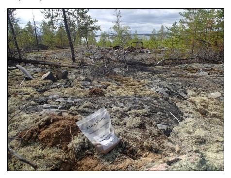
Photo 11: Soil sample collected near the scattered debris at the Assay Lab area in AEC 12.
