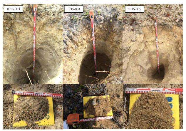
Figure 11: Test Pits dug at GD-37 showing typical consistency of material encountered
