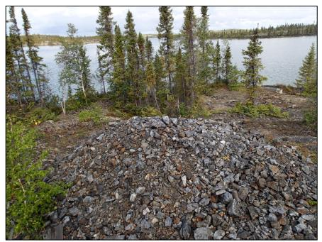
Photo 13: Waste rock / ore piles present in the Mill Area at Treacy mine site.
