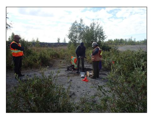
Photo 7: Hand augering within the tailings containment area (AEC 6) at Camlaren.
