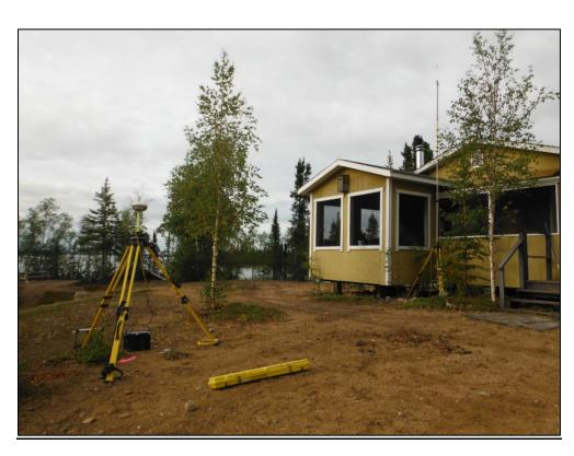
Photo 3: RTK Base Station – North Gordon Lake (GPS Coordinate: Lat: 63.089964, Long: -113.135749)
