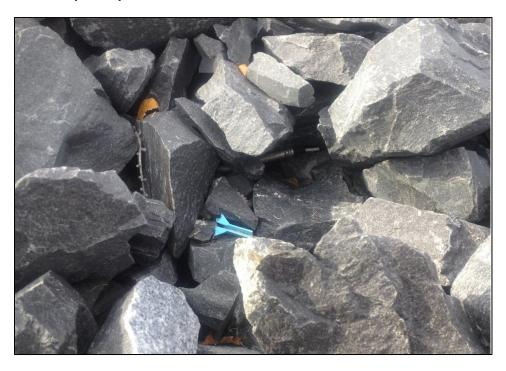
Photo D-3: Blasting caps within waste rock / ore on the eastern part of the waste rock / ore pad in AEC 17. (Source: SLR Consulting Ltd. 2013. Phase 3 Environmental Site Assessment, Kidney Pond, Northwest Territories). GPS Coordinate – Lat: 63.00713611, Long: -113.407141666
