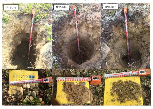
Figure 14: Photos of test pits dug at GD-65 showing the typical material encountered
